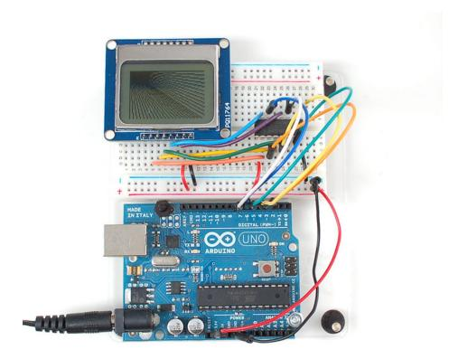
You can save some pins by connecting the CS pin to **ground** (this means you cant reuse the LCD's pins between screen updates but maybe thats OK. You can also connect the **RST** pin to the Arduino **reset** so that it will reset the screen automatically.
