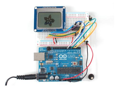
You can control the backlight, its much brighter when you connect the backlight pin to 5V (you don't need a level shifter if you are using a Nokia display from Adafruit). You can control the backlight using an Arduino pin since there is a transistor on the board.
