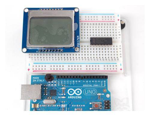
We'll start with the power lines, the system must be powered by 3.3V so red here is connected to the 3V pin from the Arduino. Ground is black.
