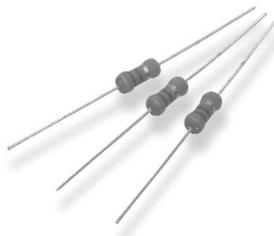
Miniature Power Oxide Resistors offer excellent performance in applications where stability and uniformity of characteristics are required. They provide smaller size for PC board application with high performance and precision to replace some wire-wound resistors and other high power resistors. Miniature metal oxide resistors withstand solvents test in accordance with MIL-STD-202E without producing mechanical or electrical damage.
