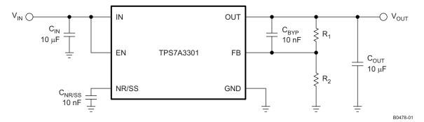
Figure 1. TPS7A3301 LDO Schematic Showing Adjustment Resistors
