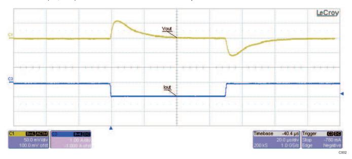
Figure 3. Load Step and Transient Response
