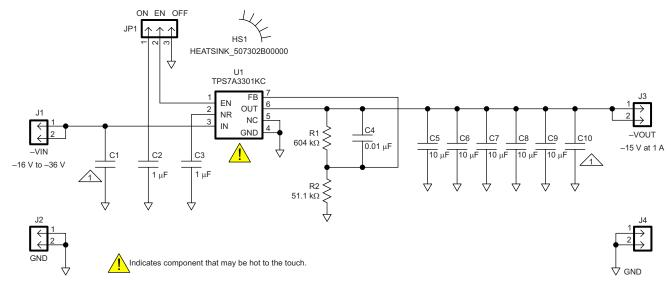
Figure 7. TPS7A3301EVM-061 Schematic
