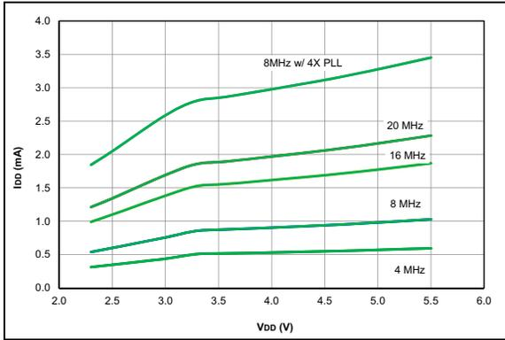
**FIGURE 37-25:**  $I_{DD}$  Typical, HS Oscillator,  $25^\circ\text{C}$ , PIC16F1764/5/8/9 Only.
