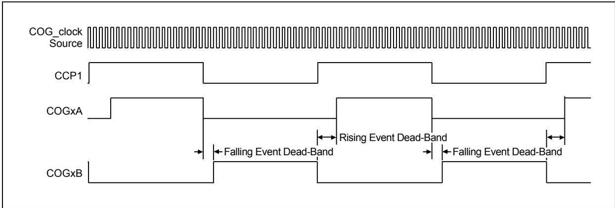
**FIGURE 27-10: HALF-BRIDGE MODE COG OPERATION WITH CCP1 AND PHASE DELAY**
