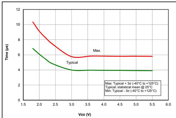
**FIGURE 37-74:** Wake From Sleep,  $V_{REGPM} = 0$ .
