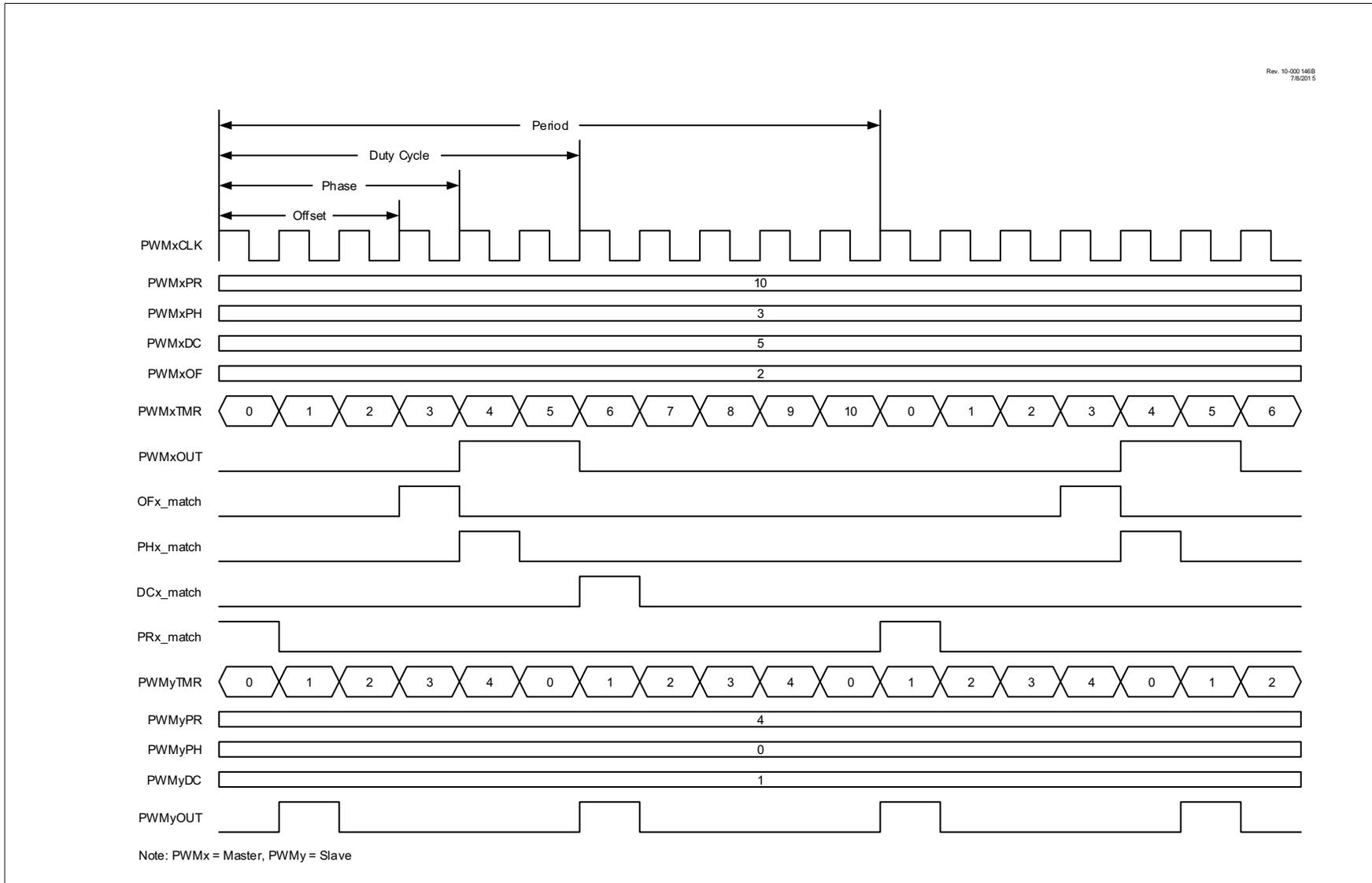
**FIGURE 26-10: ONE-SHOT SLAVE RUN MODE WITH SYNC START TIMING DIAGRAM**
