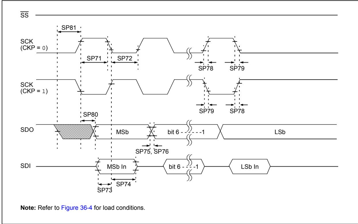
**FIGURE 36-18: SPI MASTER MODE TIMING (CKE = 1, SMP = 1)**
