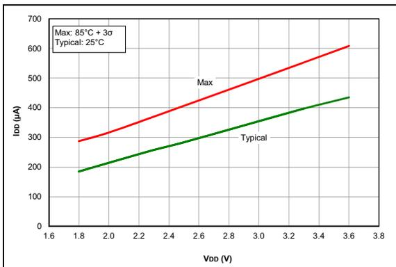
**FIGURE 37-3:**  $I_{DD}$ , XT Oscillator 4 MHz, PIC16LF1764/5/8/9 Only.
