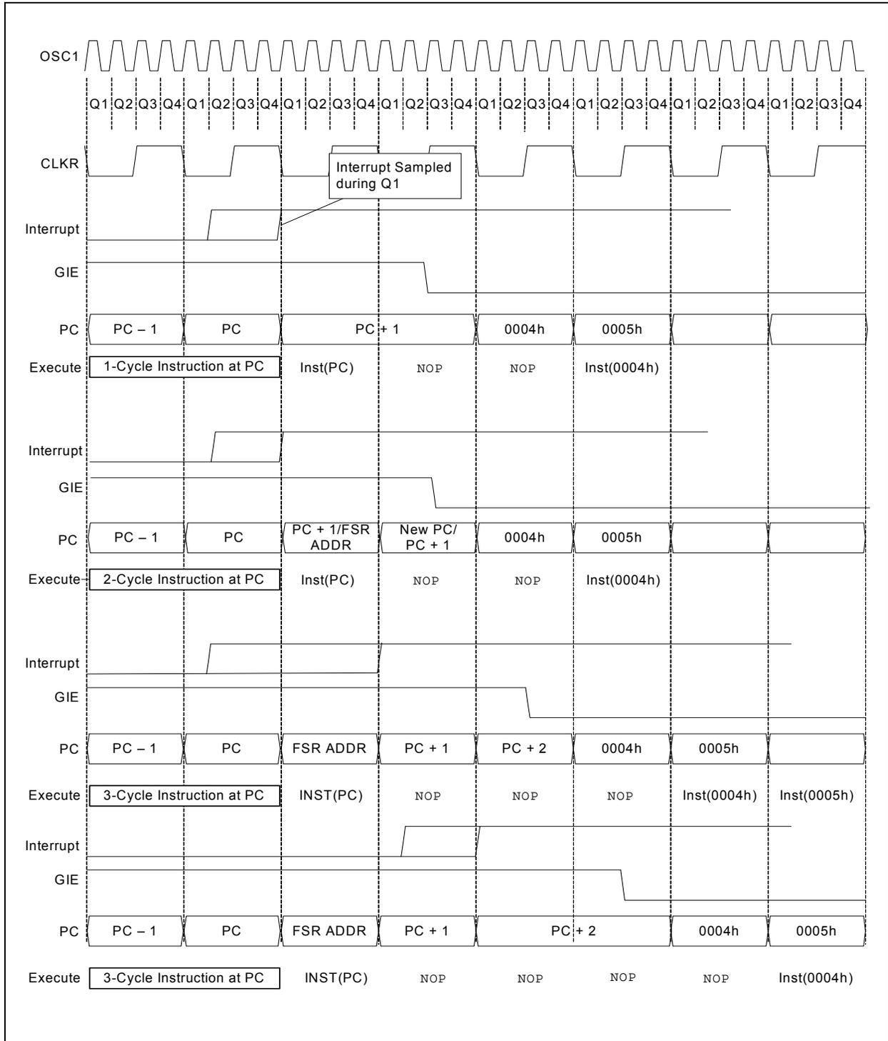
**FIGURE 7-3: INT PIN INTERRUPT TIMING**
