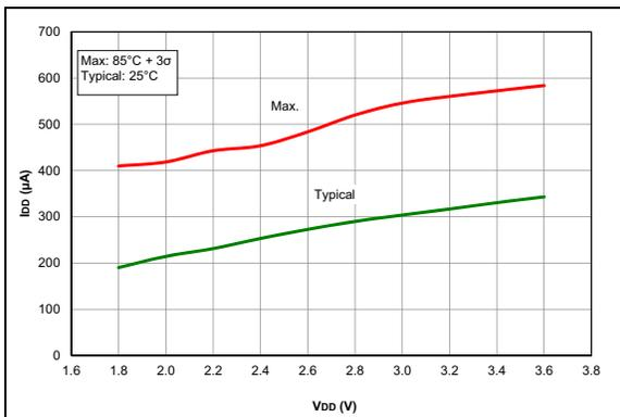
**FIGURE 37-39:**  $I_{D1}$ , Op Amp, High GBWP Mode ( $OPAxSP = 1$ ), PIC16LF1764/5/8/9 Only.
