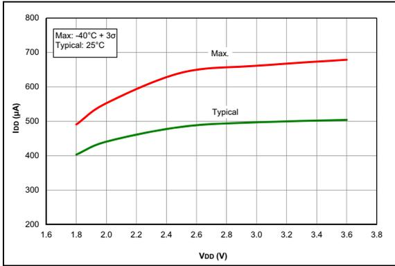
**FIGURE 37-43:**  $I_{PD}$ , Comparator, NP Mode ( $CxSP = 1$ ), PIC16LF1764/5/8/9 Only.
