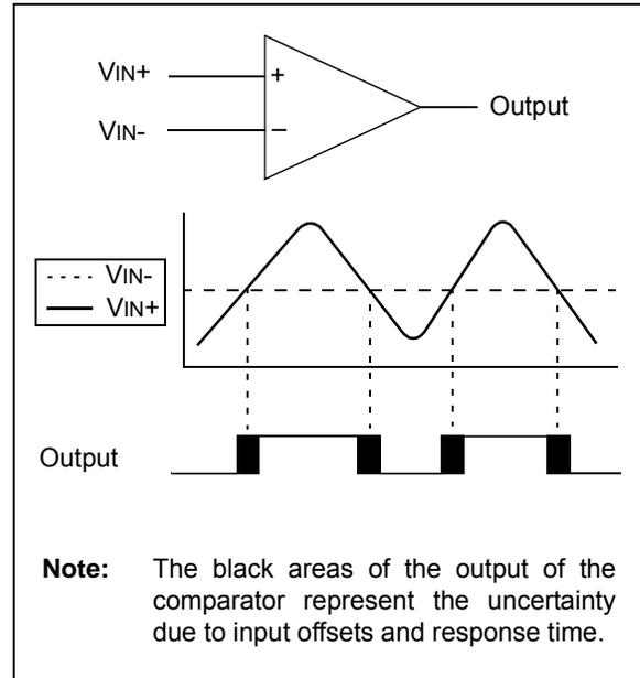
**FIGURE 19-2: COMPARATOR MODULE SIMPLIFIED BLOCK DIAGRAM**
