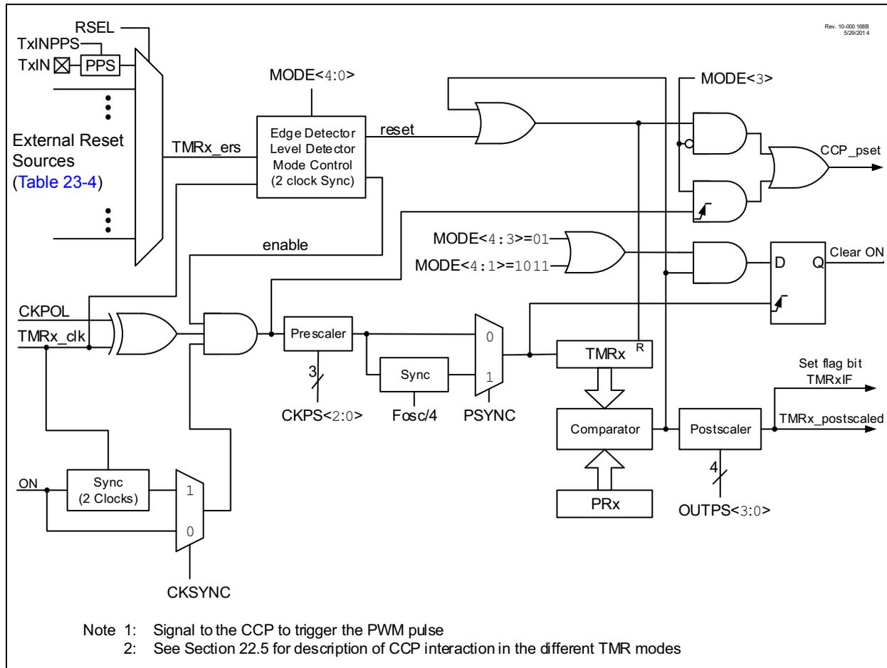
**FIGURE 23-2: TIMER2 CLOCK SOURCE BLOCK DIAGRAM**
