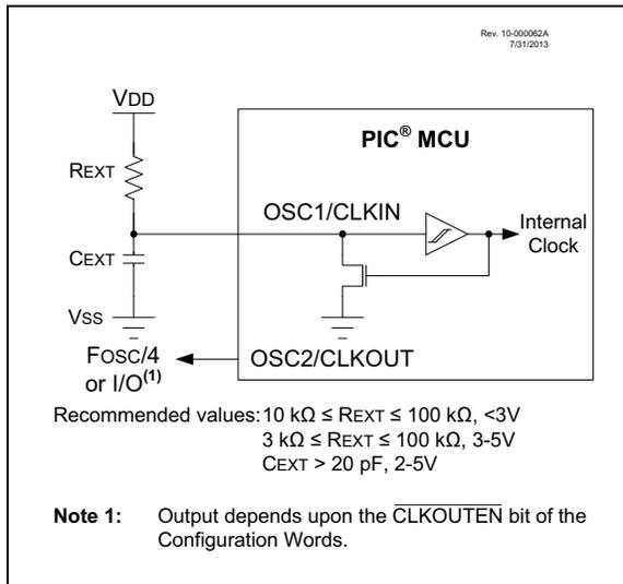
The RC oscillator frequency is a function of the supply voltage, the Resistor ( $R_{EXT}$ ) and Capacitor ( $C_{EXT}$ ) values, and the operating temperature. Other factors affecting the oscillator frequency are:
