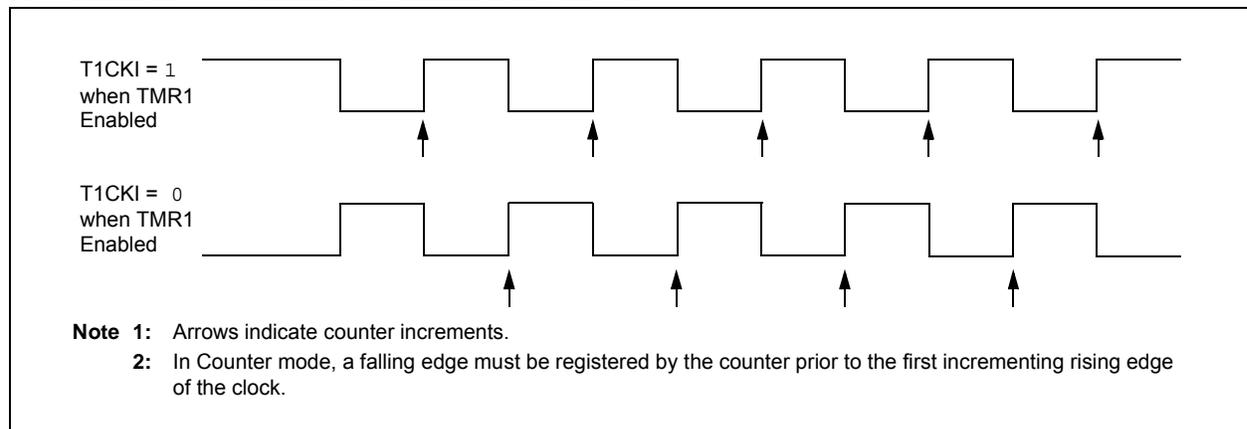
**FIGURE 22-3: TIMER1 GATE ENABLE MODE**
