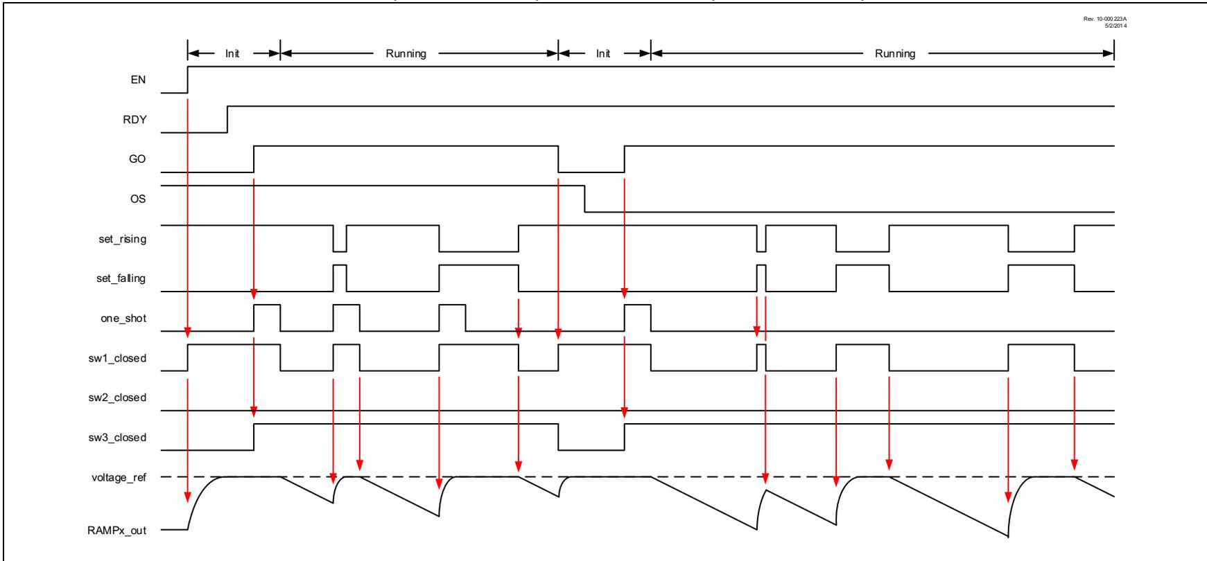
**FIGURE 30-3: ALTERNATING RISING/FALLING RAMP GENERATION TIMING DIAGRAM (OS = 0, MODE<1:0> = 01)**
