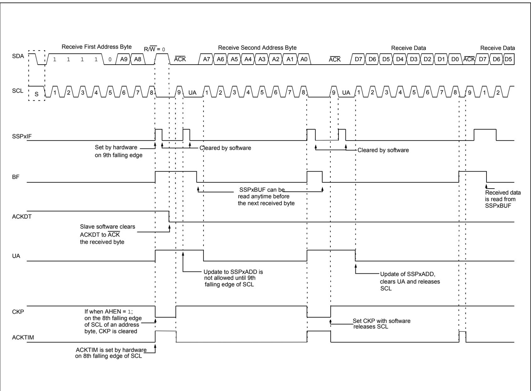
FIGURE 32-22: I<sup>2</sup>C SLAVE, 10-BIT ADDRESS, TRANSMISSION (SEN = 0, AHEN = 0, DHEN = 0)
