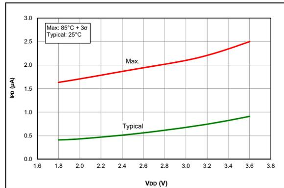
**FIGURE 37-29:**  $I_{PD}$ , Watchdog Timer (WDT), PIC16LF1764/5/8/9 Only.
