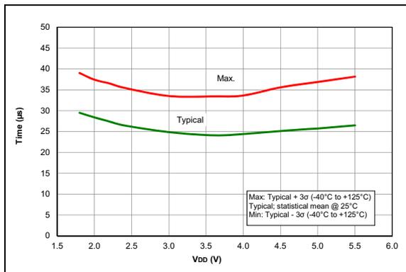
**FIGURE 37-75:** Wake From Sleep,  $V_{REGPM} = 1$ .
