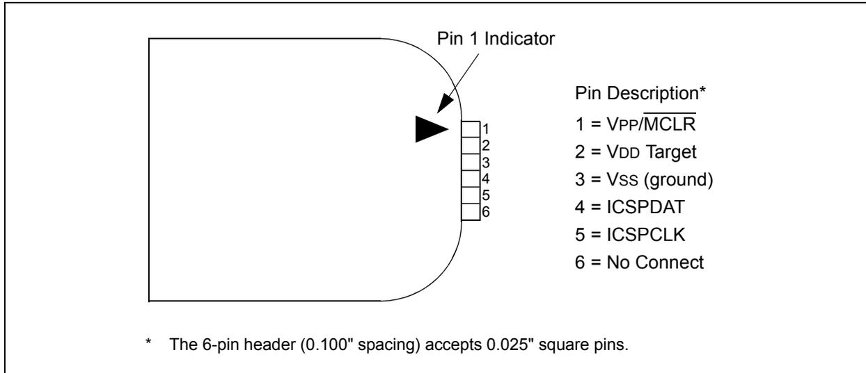
**FIGURE 34-3: TYPICAL CONNECTION FOR ICSP™ PROGRAMMING**
