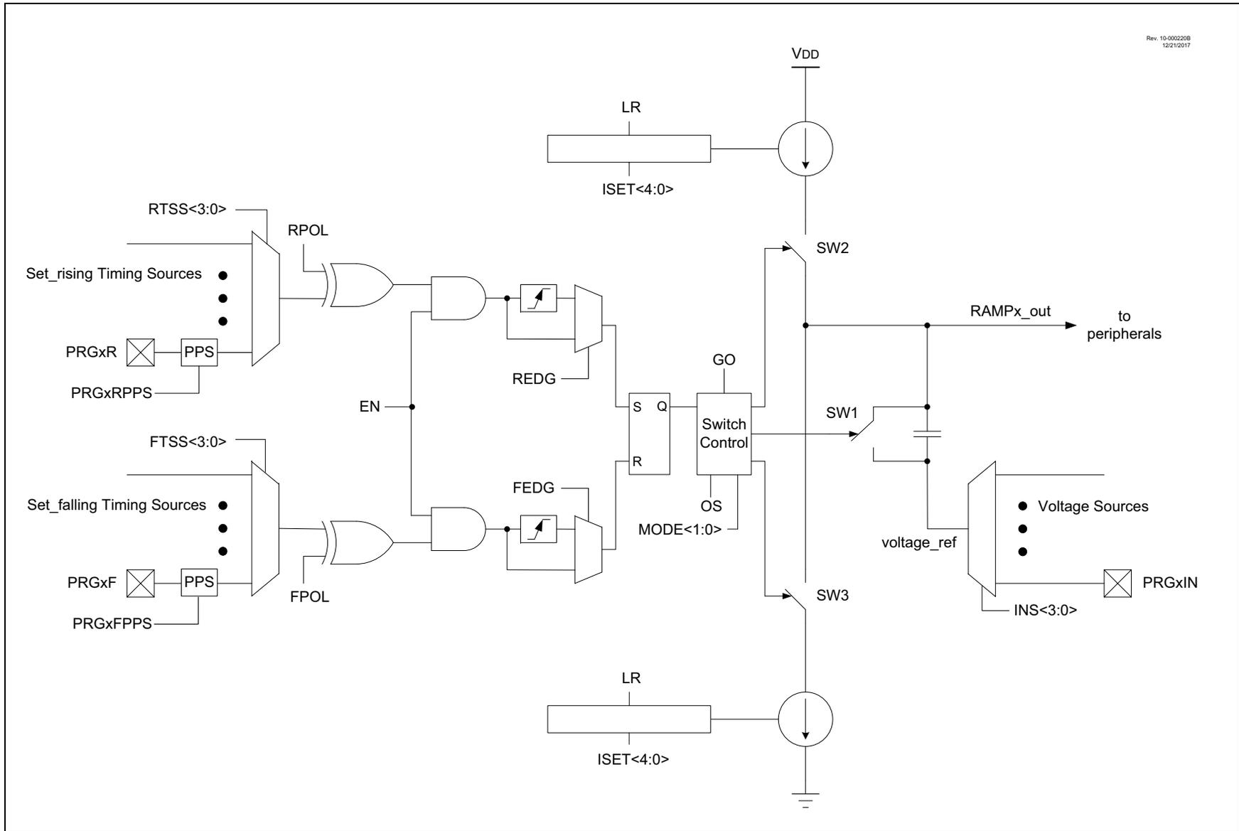
**FIGURE 30-2: SLOPE COMPENSATION (FALLING RAMP) TIMING DIAGRAM (MODE<1:0> = 00)**
