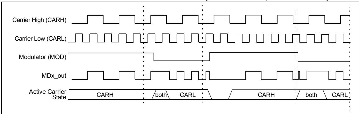
**FIGURE 31-5: CARRIER LOW SYNCHRONIZATION (MDCHSYNC = 0, MDCLSYNC = 1)**
