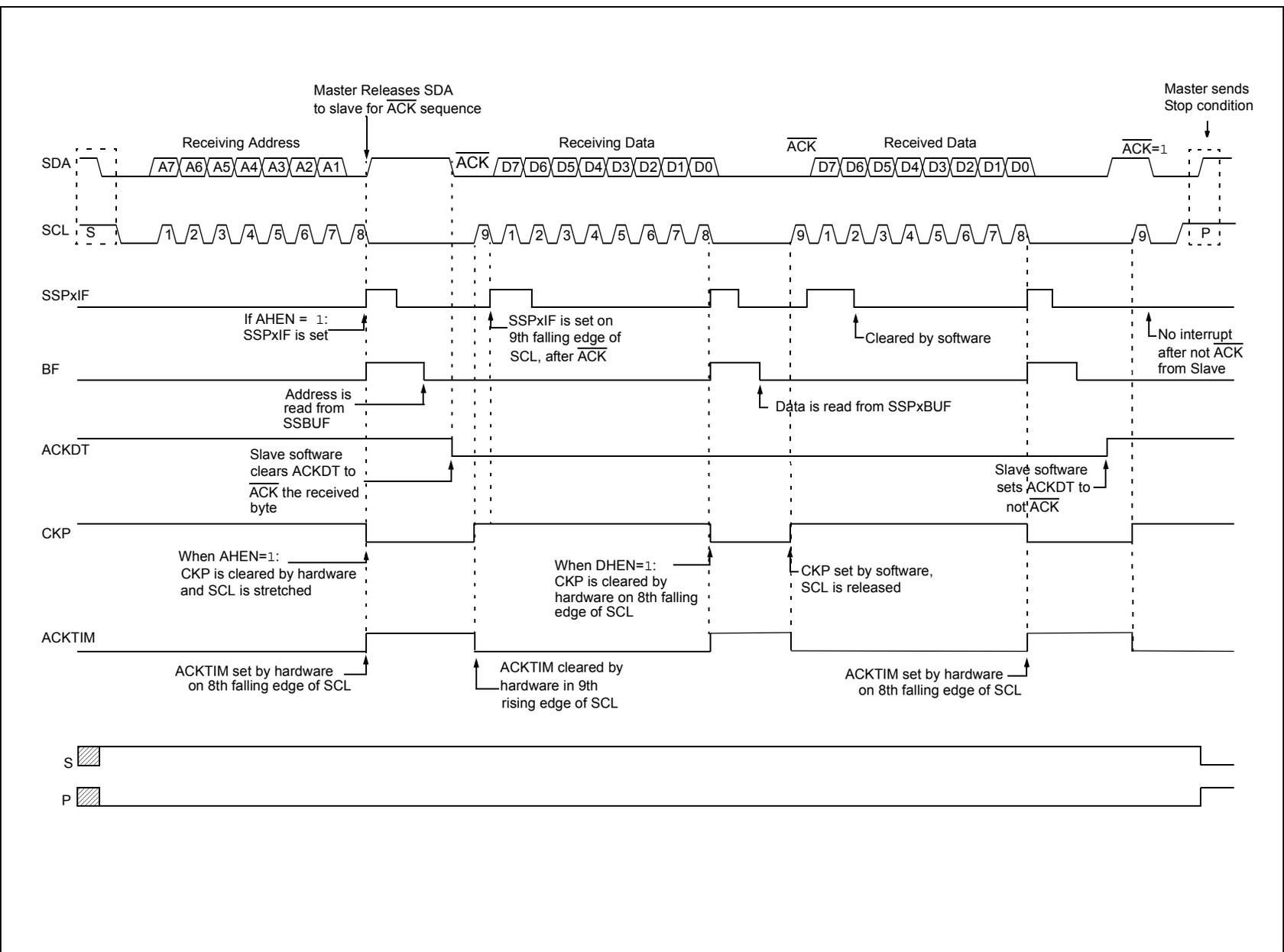
FIGURE 32-17: I<sup>2</sup>C SLAVE, 7-BIT ADDRESS, RECEPTION (SEN = 1, AHEN = 1, DHEN = 1)
