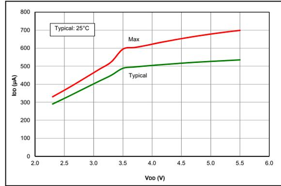
**FIGURE 37-4:**  $I_{DD}$ , XT Oscillator, 4 MHz, PIC16F1764/5/8/9 Only.
