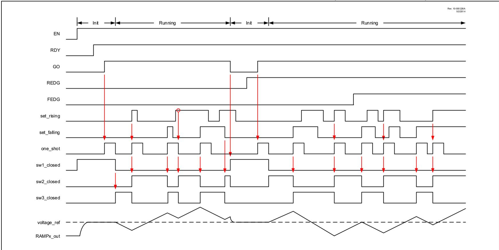
**FIGURE 30-5: RISING RAMP GENERATION TIMING DIAGRAM (MODE<1:0> = 10)**
