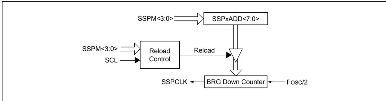
**Note:** Values of 0x00, 0x01 and 0x02 are not valid for SSPxADD when used as a Baud Rate Generator for I<sup>2</sup>C; this is an implementation limitation.
