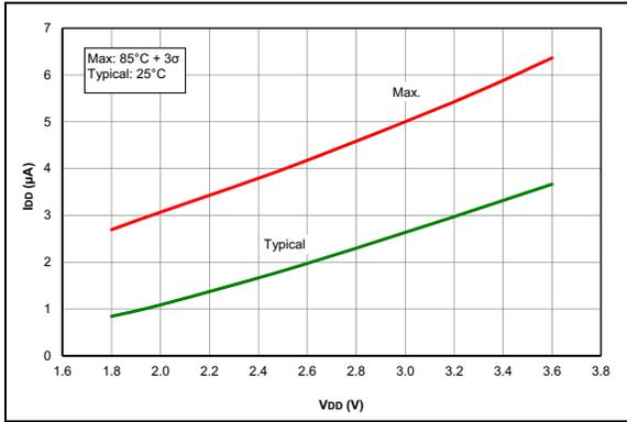
**FIGURE 37-37:**  $I_{D1}$ , Timer1 Oscillator,  $F_{OSC} = 32\text{ kHz}$ , PIC16LF1764/5/8/9 Only.
