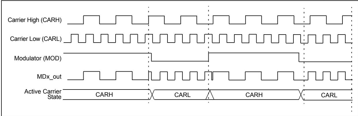
**FIGURE 31-6: FULL SYNCHRONIZATION (MDCHSYNC = 1, MDCLSYNC = 1)**
