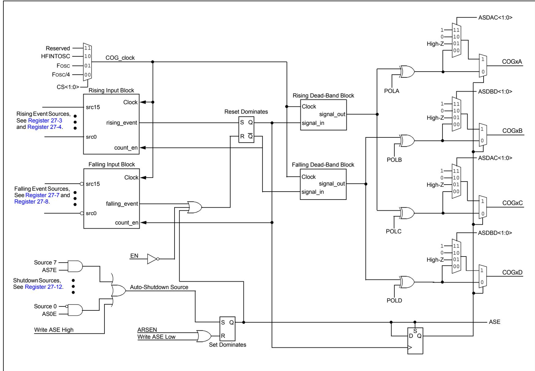
**FIGURE 27-6: SIMPLIFIED COG BLOCK DIAGRAM (PUSH-PULL MODE, MD<2:0> = 5)**
