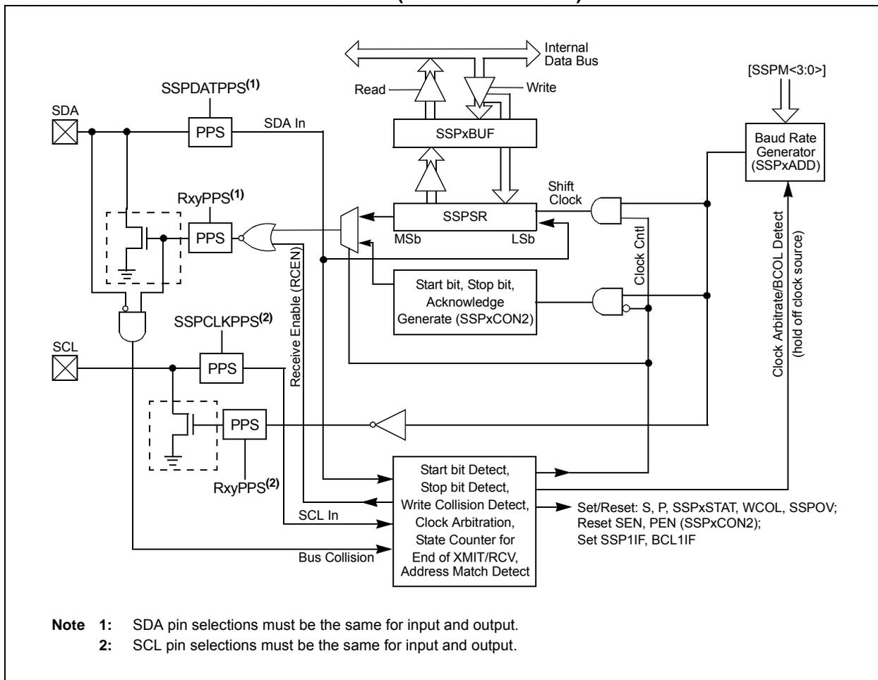
**FIGURE 32-3: MSSP BLOCK DIAGRAM (I<sup>2</sup>C SLAVE MODE)**
