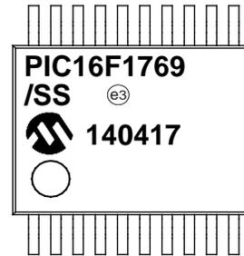
20-Lead SOIC (7.50 mm)
