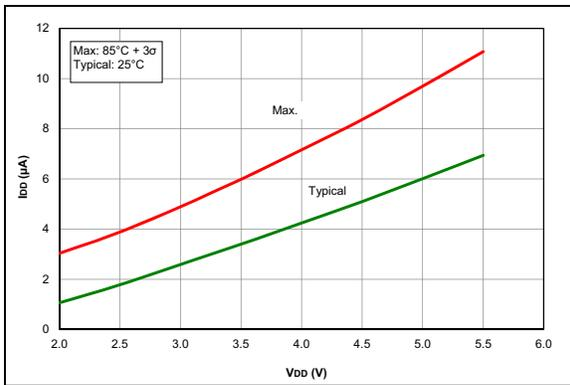
**FIGURE 37-38:**  $I_{D1}$ , Timer1 Oscillator,  $F_{OSC} = 32\text{ kHz}$ , PIC16F1764/5/8/9 Only.
