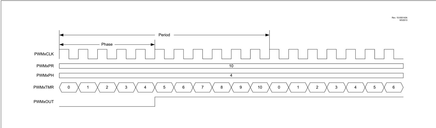
**FIGURE 26-6: TOGGLE ON MATCH PWMx MODE TIMING DIAGRAM**
