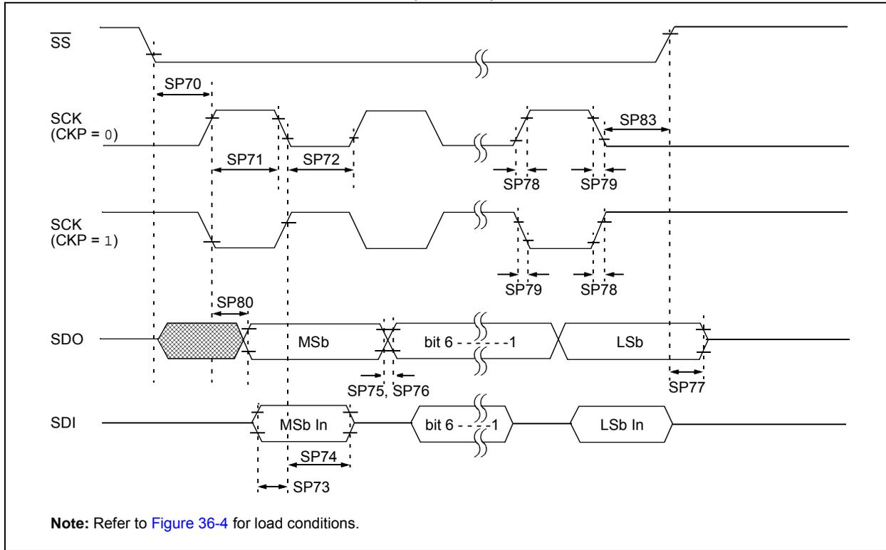
**FIGURE 36-20: SPI SLAVE MODE TIMING (CKE = 1)**
