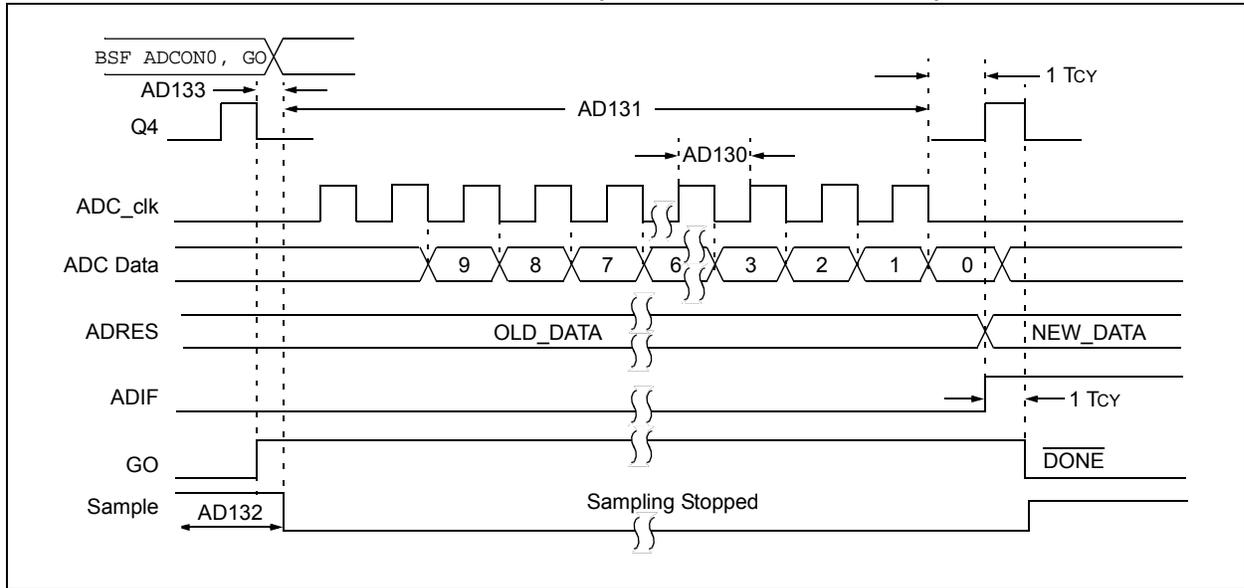
**FIGURE 36-14: ADC CONVERSION TIMING (ADC CLOCK FROM FRC)**
