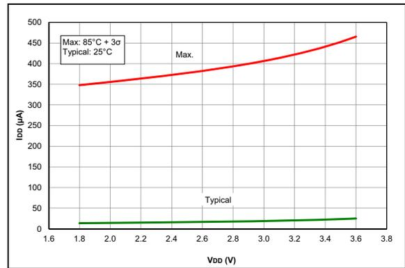
**FIGURE 37-41:**  $I_{D1}$ , ADC Non-Converting, PIC16LF1764/5/8/9 Only.
