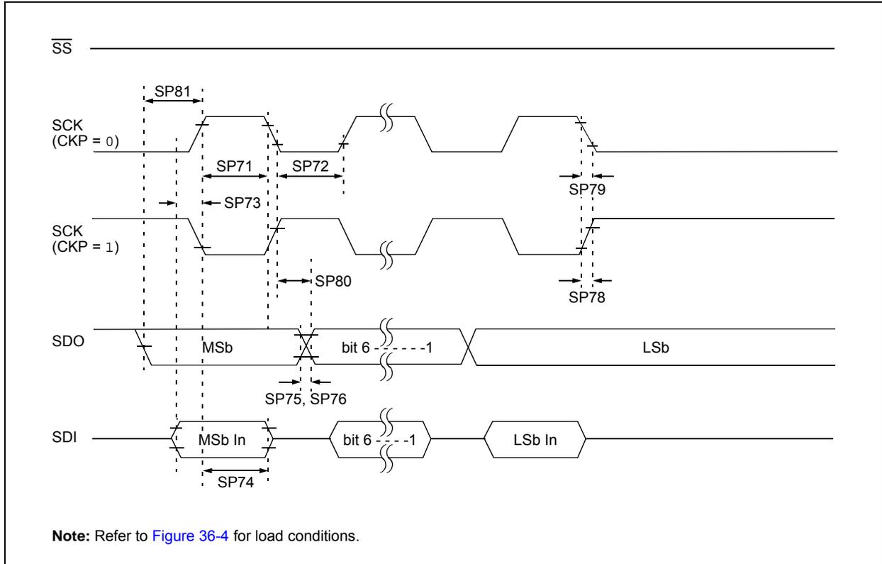
**FIGURE 36-19: SPI SLAVE MODE TIMING (CKE = 0)**
