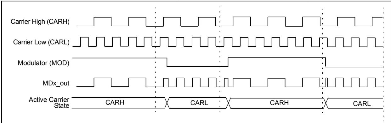
**FIGURE 31-4: CARRIER HIGH SYNCHRONIZATION (MDCHSYNC = 1, MDCLSYNC = 0)**
