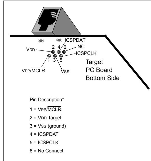
Another connector often found in use with the PICkit™ programmers is a standard 6-pin header with 0.1 inch spacing. Refer to [Figure 34-2](#).
