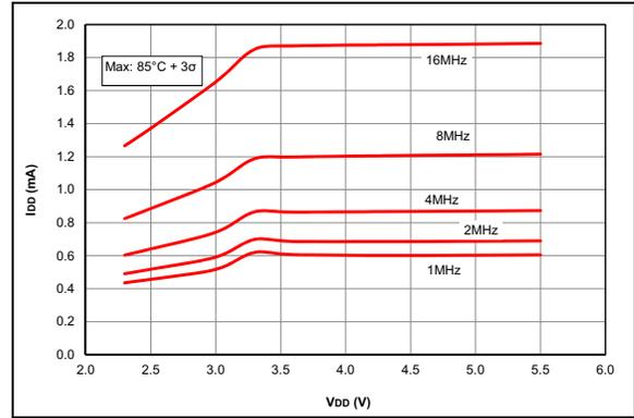
**FIGURE 37-22:**  $I_{DD}$  Maximum, HFINTOSC Mode, PIC16LF1764/5/8/9 Only.
