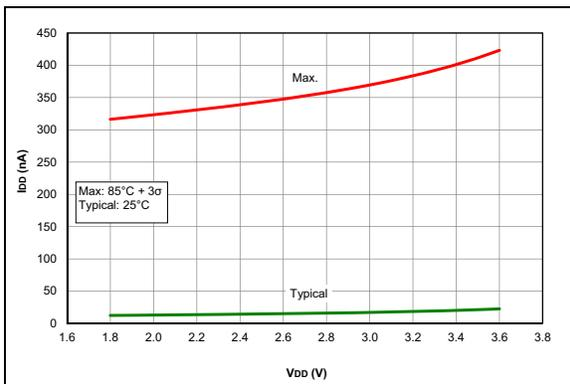
**FIGURE 37-27:**  $I_{PD}$  Base, LP Sleep Mode, PIC16LF1764/5/8/9 Only.
