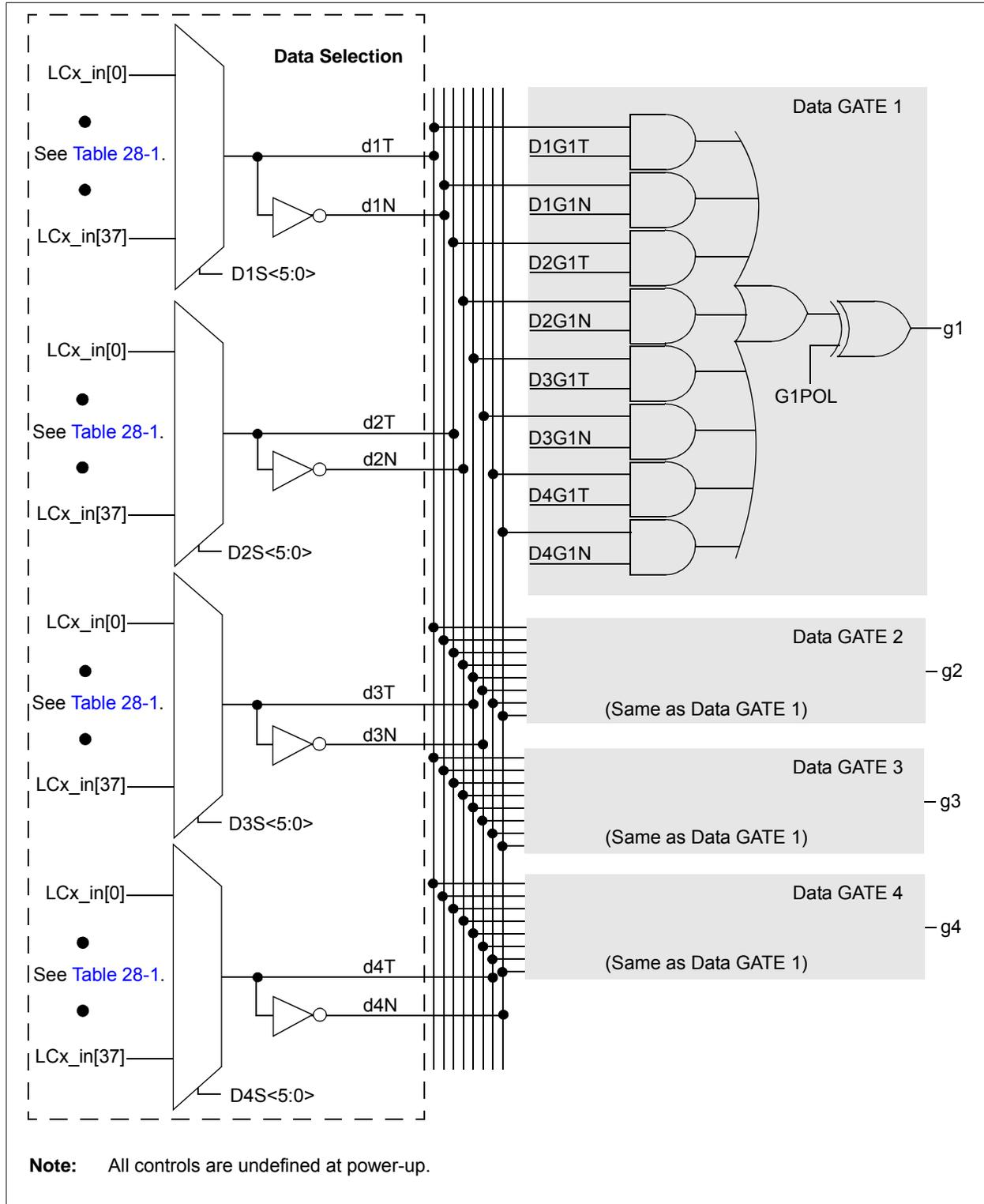
**FIGURE 28-3: PROGRAMMABLE LOGIC FUNCTIONS**
