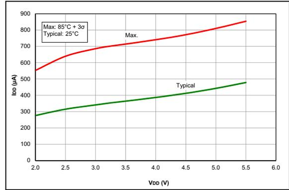
**FIGURE 37-40:**  $I_{D1}$ , Op Amp, High GBWP Mode ( $OPAxSP = 1$ ), PIC16F1764/5/8/9 Only.
