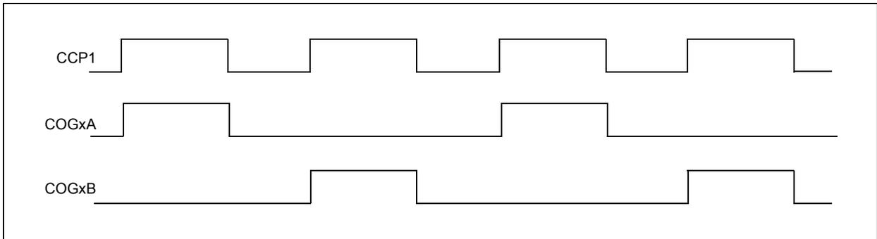
**FIGURE 27-12: FULL-BRIDGE FORWARD MODE COG OPERATION WITH CCP1**
