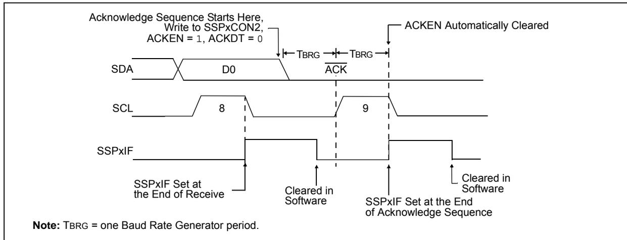
**FIGURE 32-31: STOP CONDITION RECEIVE OR TRANSMIT MODE**
