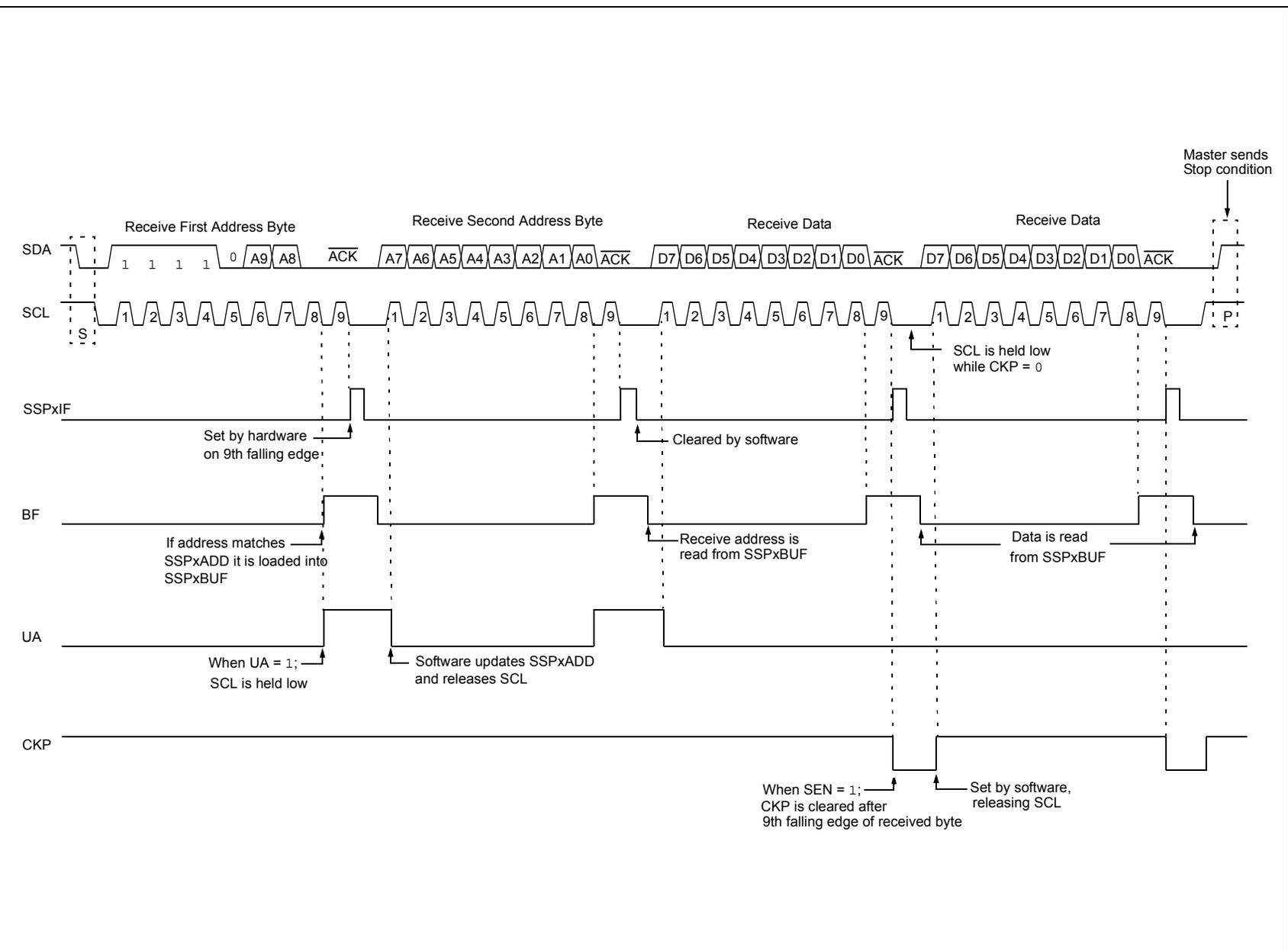
FIGURE 32-21: I<sup>2</sup>C SLAVE, 10-BIT ADDRESS, RECEPTION (SEN = 0, AHEN = 1, DHEN = 0)
