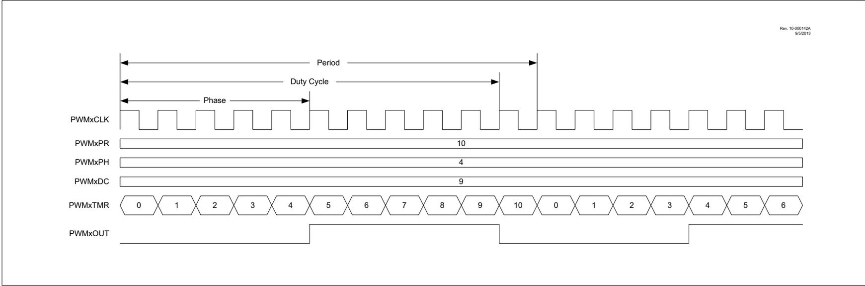
**FIGURE 26-5: SET ON MATCH PWMx MODE TIMING DIAGRAM**
