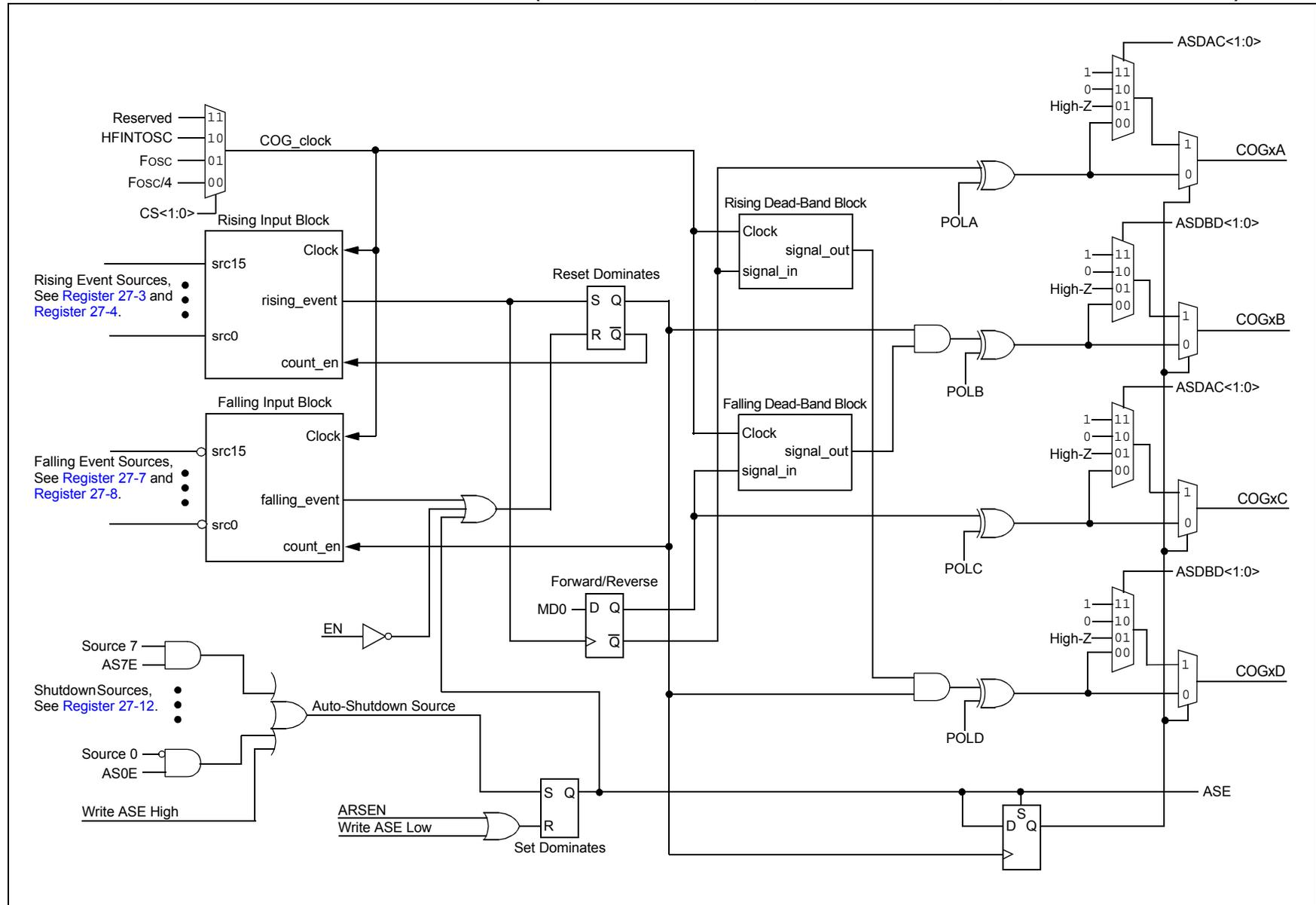
**FIGURE 27-5: SIMPLIFIED COG BLOCK DIAGRAM (HALF-BRIDGE MODE, MD<2:0> = 4)**
