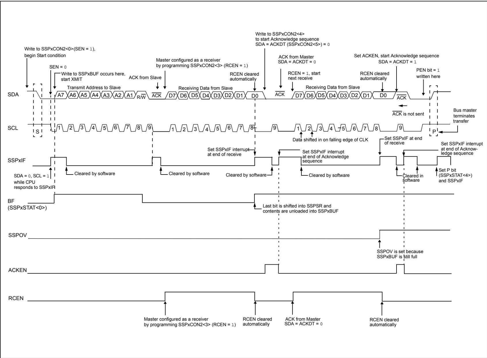
FIGURE 32-29: I<sup>2</sup>C MASTER MODE WAVEFORM (RECEPTION, 7-BIT ADDRESS)
