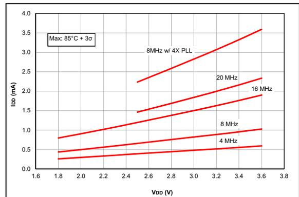
**FIGURE 37-24:**  $I_{DD}$  Maximum, HS Oscillator, PIC16LF1764/5/8/9 Only.
