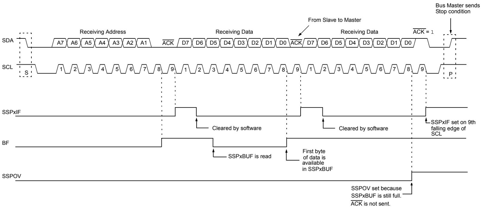
FIGURE 32-16: I<sup>2</sup>C SLAVE, 7-BIT ADDRESS, RECEPTION (SEN = 0, AHEN = 1, DHEN = 1)
