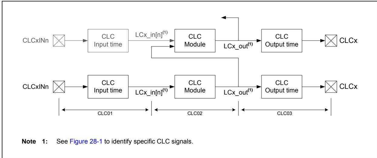
**TABLE 36-14: CONFIGURATION LOGIC CELL (CLC) CHARACTERISTICS**
