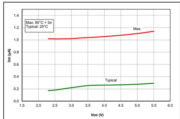
**FIGURE 37-42:**  $I_{D1}$ , ADC Non-Converting, PIC16F1764/5/8/9 Only.
