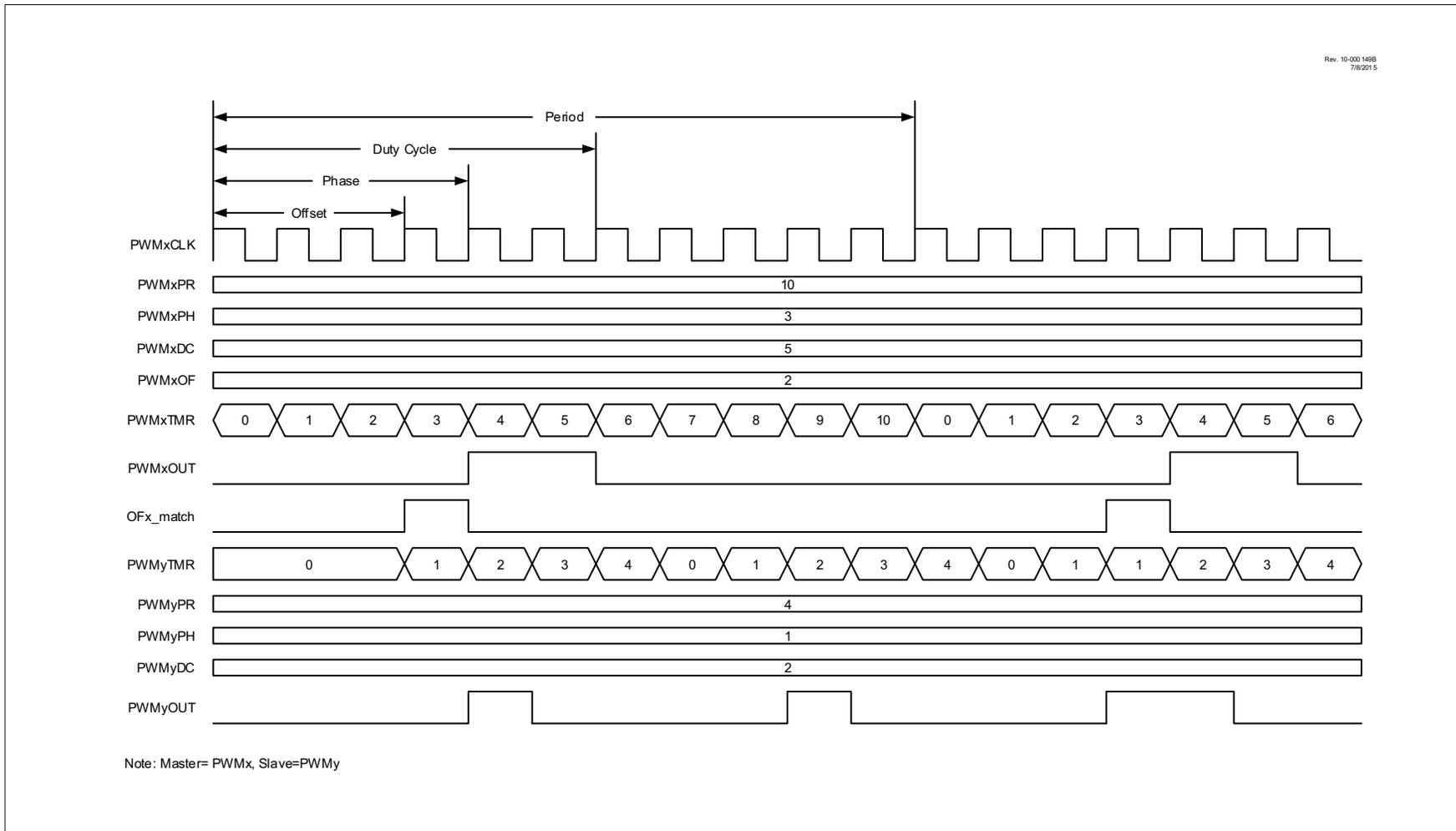
**FIGURE 26-12: OFFSET MATCH ON INCREMENTING TIMER TIMING DIAGRAM**
