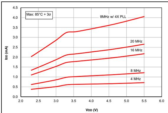
**FIGURE 37-26:**  $I_{DD}$  Maximum, HS Oscillator, PIC16F1764/5/8/9 Only.
