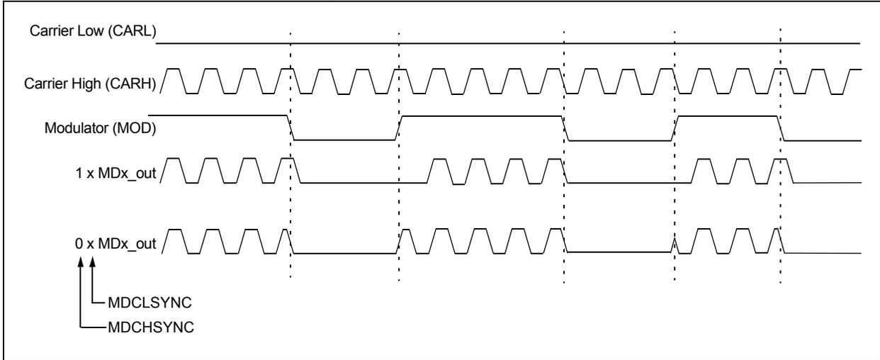
**FIGURE 31-3: NO SYNCHRONIZATION (MDCHSYNC = 0, MDCLSYNC = 0)**
