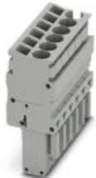
Plug, Connection method: Spring-cage connection, Number of positions: 1, Cross section: 0.08 mm<sup>2</sup> - 4 mm<sup>2</sup>, AWG: 28 - 12, Width: 5.2 mm, Height: 39 mm, Color: gray
