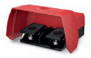
Two Stage Operation-Press Pedal to change the state of the first set of contacts. Continue to press further to change the second set of contacts.
