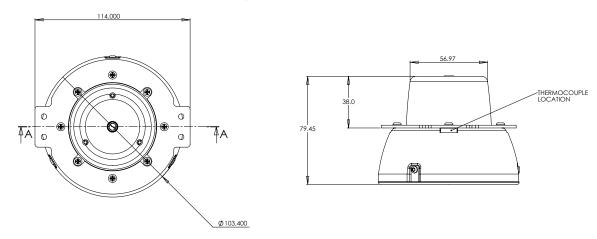
The operating temperature of the Cree LED Module LMR4 is between 0 °C and 50 °C. The lifetime and performance estimates described in this document apply only if the product's Thermal Management Guidelines (below) are adhered to and no modifications are made except as described in this document.
