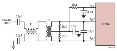
T1: MA/COM MABA-007159-000000 T2: COILCRAFT WBC1-1TL RESISTORS, CAPACITORS ARE 0402 PACKAGE SIZE
