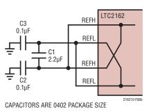
Figure 8b. Alternative REFH/REFL Bypass Circuit
