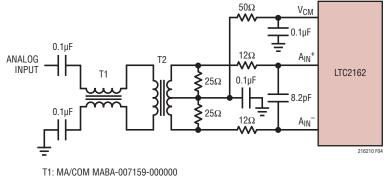
T2: COILCRAFT WBC1-1TL RESISTORS, CAPACITORS ARE 0402 PACKAGE SIZE
