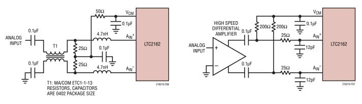
Figure 6. Recommended Front End Circuit for Input Frequencies Above 250MHz Figure 7. Front End Circuit Using a High Speed Differential Amplifier
