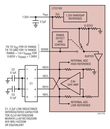
Figure 8a. Reference Circuit
