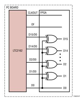
Figure 16. Unrandomizing a Randomized Digital Output Signal
