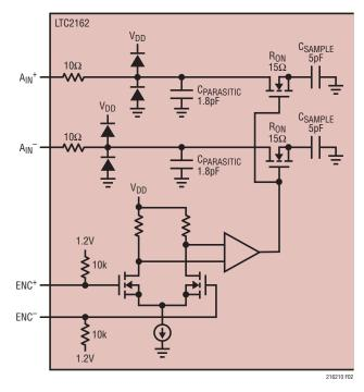
Figure 2. Equivalent Input Circuit
