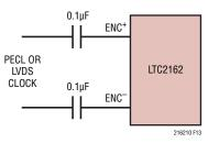
Figure 13. PECL or LVDS Encode Drive
