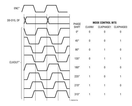
Figure 14. Phase-Shifting CLKOUT
