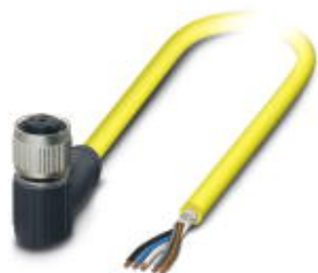
Sensor/actuator cable, 5-position, PVC, yellow, shielded, free cable end, on Socket angled M12 SPEEDCON, coding: A, cable length: 10 m
