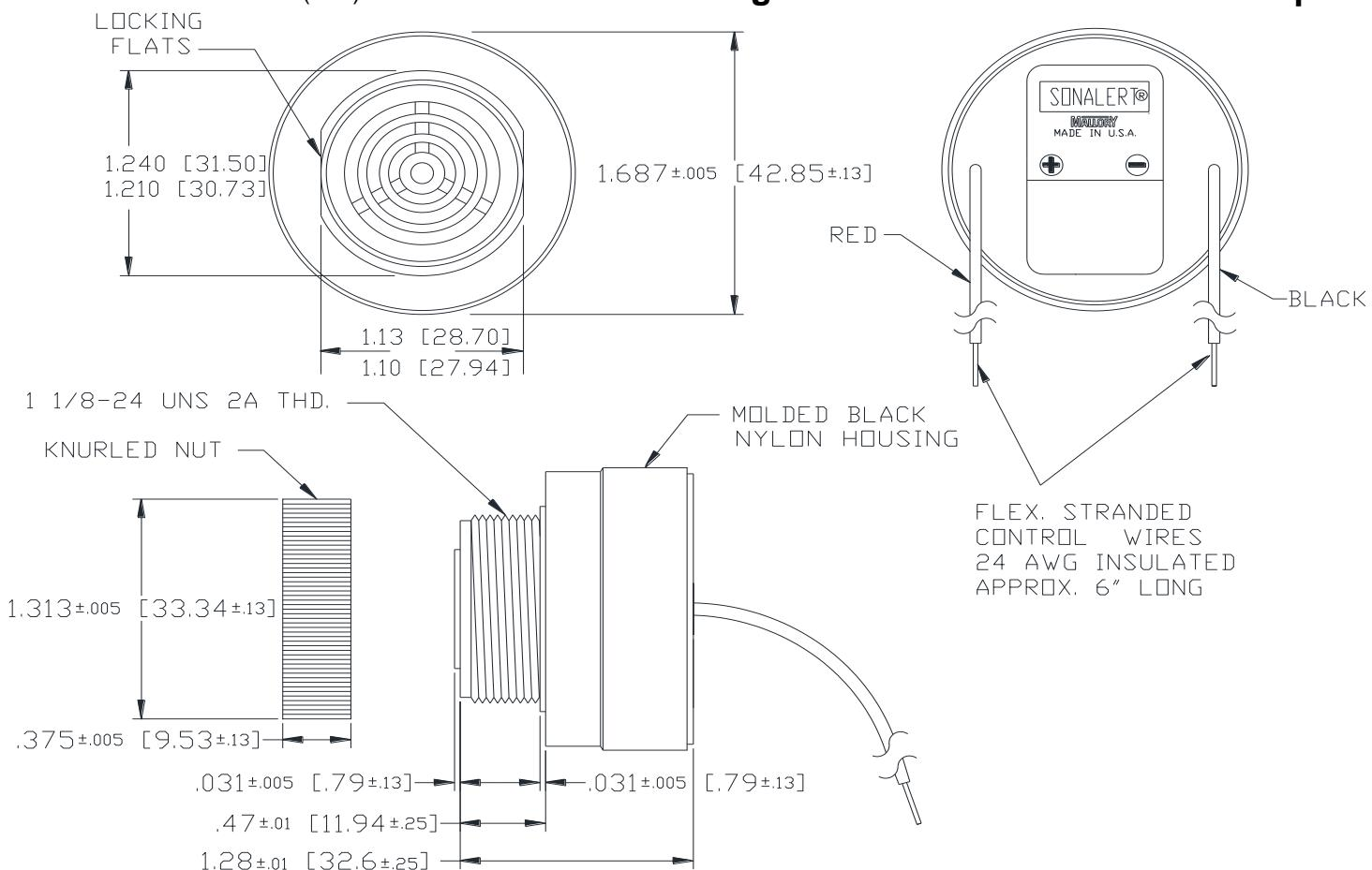
NOTE: MOUNTING- REMOVE BLACK PLASTIC NUT AND INSERT THREADED FRONT THROUGH 1.25" HOLE PUNCHED IN PANEL, IF ORIENTATION IS NEEDED, NOTE LOCKING FLATS ON DRAWING. SCREW NUT BACK ON. DO NOT OVERTIGHTEN.
