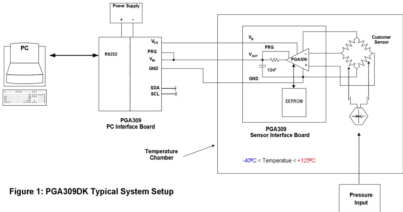
**Figure 1: PGA309DK Typical System Setup**
