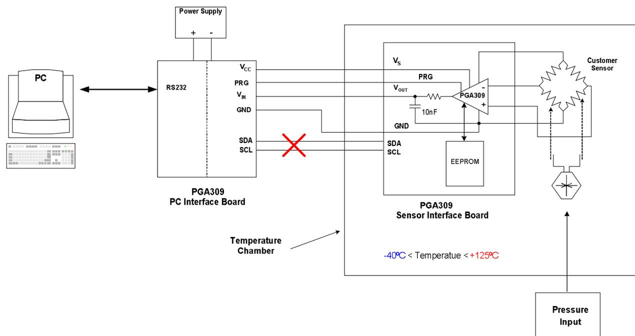
Figure 46: Use One-Wire (PRG) Interface for Temperature Calibration
