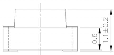
For reflow soldering
