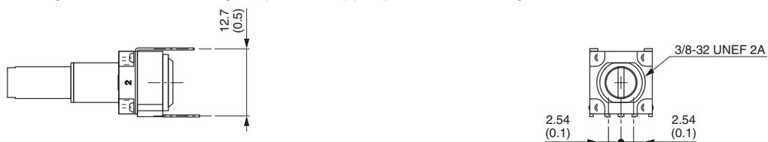
Dual modules, single shaft, PC pins with front support plates, imperial bushing and shaft
