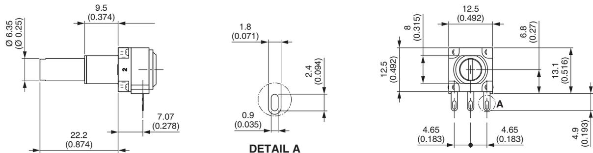
Single module, single shaft, vertical mounting, PC pins with support plate, metric bushing and shaft
