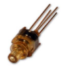
The HFD3180-203 use a high-performance GaAs PIN photo-detector packaged with a transimpedance amplifier designed to meet performance requirements for data rates up to 4.25Gbps data communication over multi-mode optical fiber at 850nm. Applications include Ethernet, Fiber Channel and ATM protocols. The optical assembly is designed to interface either 50mm or 62.5mm multi-mode fiber.
