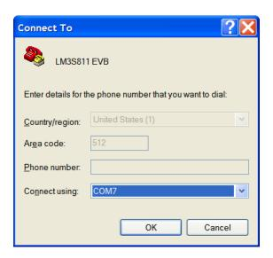
**5.** Use the Properties dialog box to set the Port Settings. The quickstart application sends data at 115200 baud, 8 data bits, no parity, 1 stop bit, and no flow-control. Click OK.
