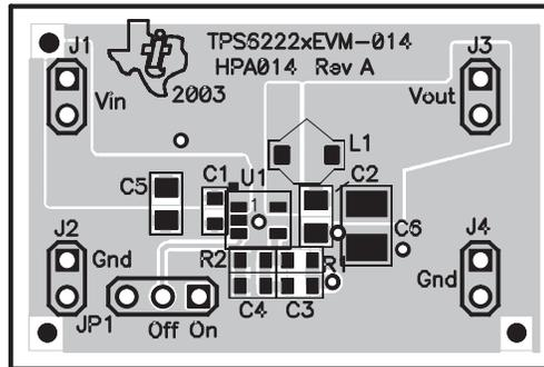
Figure 3–2. Top Layer Routing
