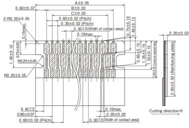
$\ensuremath{\mbox{\ensuremath{\mbox{\sc WCut}}}\xspace}$  FPC from the copper foil side to the reinforcing plate side
