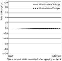
Characteristics were measured after applying a shock of 490 m/s<sup>2</sup> to the test piece 3 times each in 6 directions along 3 axes.
