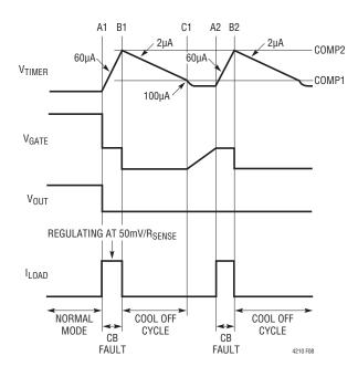
Figure 8. Automatic Retry After Overcurrent Fault
