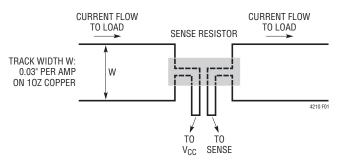
Figure 1. Making PCB Connections to the Sense Resistor
