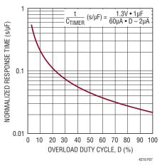
Figure 7. Circuit Breaker Timer Response for Intermittent Overload
