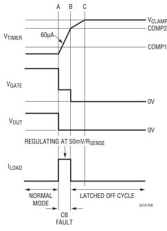
Figure 9. Latchoff After Overcurrent Fault
