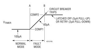
Figure 5. A Continuous Fault Timing
