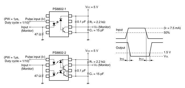
Remark C<sub>L</sub> is approximately 15 pF which includes probe and stray wiring capacitance.
