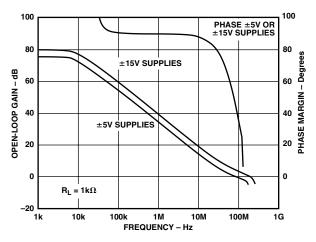
TPC 10. Open-Loop Gain and Phase Margin vs. Frequency
