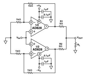
Figure 5. Parallel Amp Configuration
