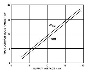
TPC 1. Common-Mode Voltage Range vs. Supply Voltage
