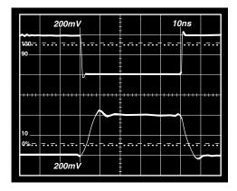
TPC 29. Inverter Small Signal Pulse Response  $\pm$  15  $V_{\rm S}$ ,  $C_{\rm F}$  = 1 pF,  $R_{\rm L}$  = 1500  $\Omega$
