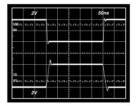
TPC 26. Inverter Large Signal Pulse Response  $\pm 5~V_S$ ,  $C_F = 1~pF$ ,  $R_L = 1~k\Omega$
