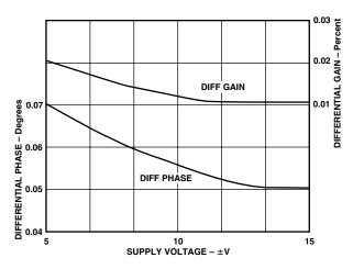
TPC 20. Differential Gain and Phase vs. Supply Voltage
