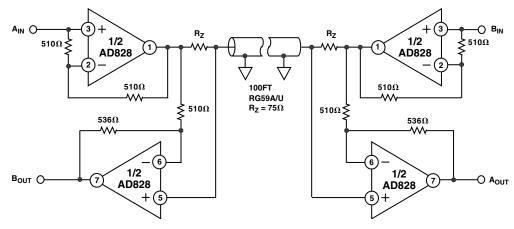
Figure 6. Bidirectional Transmission CKT
