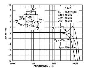
TPC 19. Closed-Loop Gain vs. Frequency
