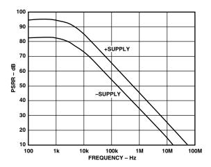
TPC 12. Power Supply Rejection vs. Frequency
