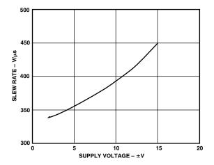
TPC 5. Slew Rate vs. Supply Voltage
