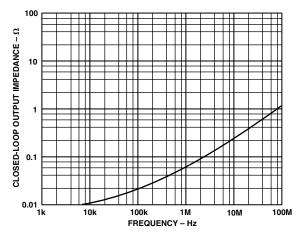
TPC 6. Closed-Loop Output Impedance vs. Frequency
