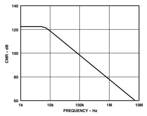
TPC 13. Common-Mode Rejection vs. Frequency
