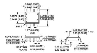
CONTROLLING DIMENSIONS ARE IN MILLIMETERS; INCH DIMENSIONS (IN PARENTHESES) ARE ROUNDED-OFF MILLIMETER EQUIVALENTS FOR REFERENCE ONLY AND ARE NOT APPROPRIATE FOR USE IN DESIGN COMPLIANT TO JEDEC STANDARDS MS-012 AA
