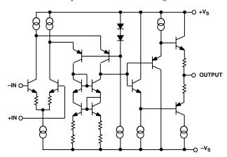
Figure 4. Simplified Schematic
