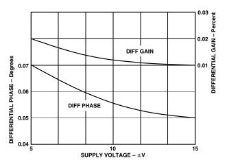
Figure 2. Differential Phase vs. Supply Voltage
