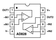
The AD828 is fully specified for operation with a single 5 V power supply and with dual supplies from  $\pm 5$  V to  $\pm 15$  V. This power supply flexibility, coupled with a very low supply current of 15 mA and excellent ac characteristics under all power supply conditions, make the AD828 the ideal choice for many demanding yet power-sensitive applications.
