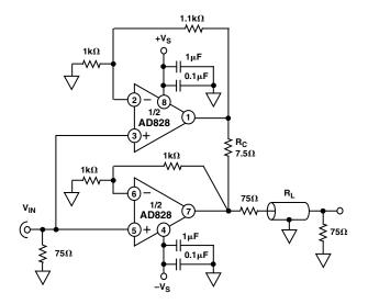
Figure 10. Low Distortion Amplifier
