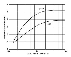
TPC 11. Open-Loop Gain vs. Load Resistance
