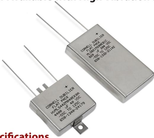
Encased in rugged stainless steel, the MLS is perfect for high reliability military systems and applications operating above 85 °C. For our highest performing 125 °C Flatpacks, choose type HVMLS available in a special stainless steel case for high vibration applications up to 50g. Specify type HRMLS for high reliability Flatpacks which are subjected to MIL level burn-in processes to ensure established reliability.
