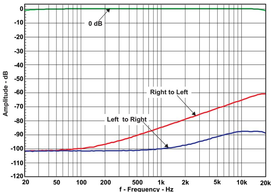
**Figure 16. Channel Separation**
