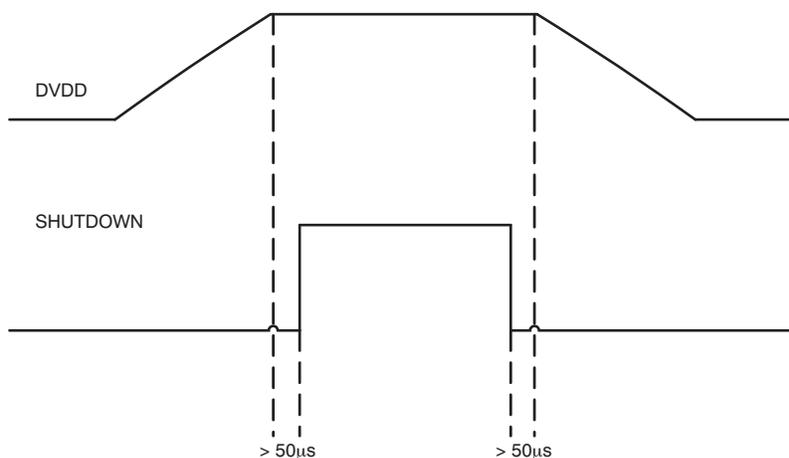
**Figure 4. Power-Up/Down Sequence**
