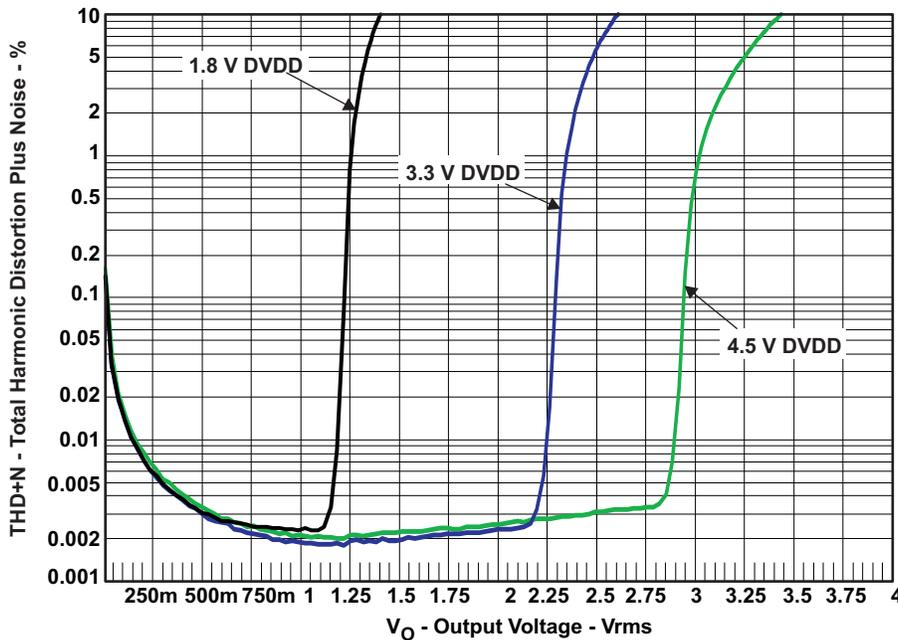
Figure 9. THD+N vs Voltage (100-Ω load) Linear Scale
