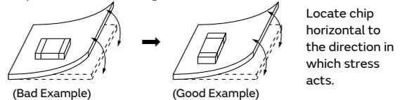
**[Chip Mounting Close to Board Separation Point]**
