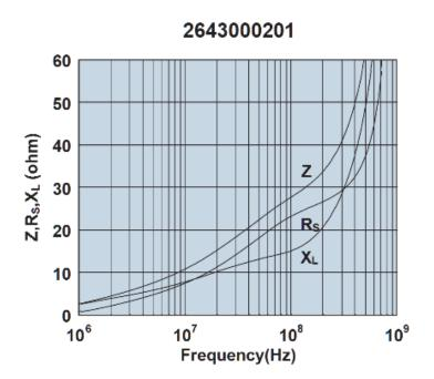
Impedance, reactance, and resistance vs. frequency.
