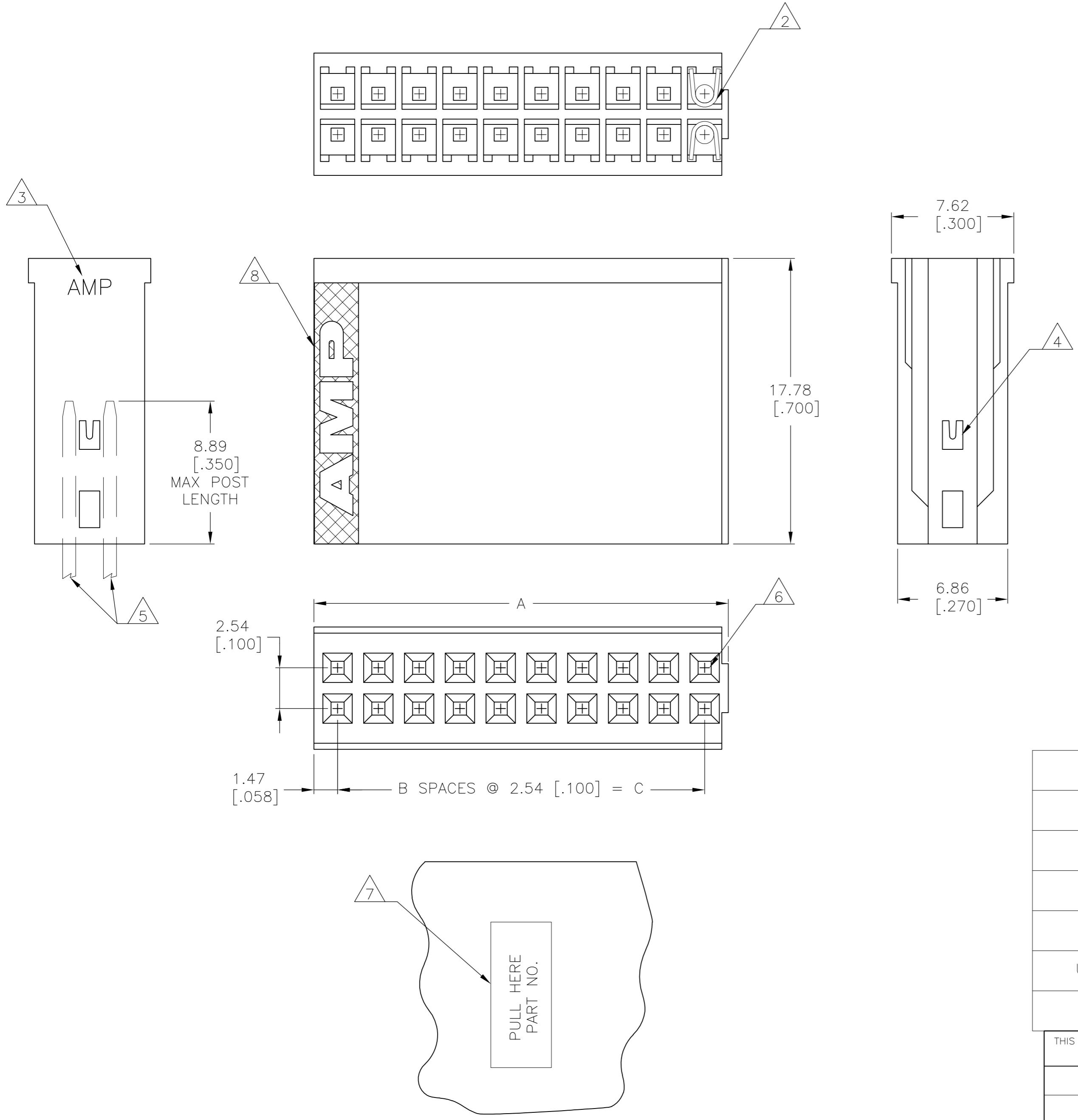
1 PULL ON HOUSING TO REMOVE FROM POSTS. DO NOT CONFIN THE CONDUCTORS OR PULL ON THE CONDUCTORS DURING REMOVAL ACTION.
