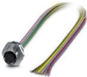
Flush-type connector, Universal, 12-position, Socket, M12, A-coded, Front mounting, M16 x 1.5, Individual wires, cable length: 0.5 m, 0.14 mm², TPE litz wire
