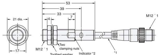
\*1. 6-dia. vinyl-insulated round cable (flame retardant), Standard length; 300 mm
