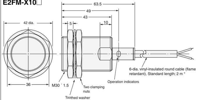
\* 6-dia. vinyl-insulated round cable with 2 conductors
