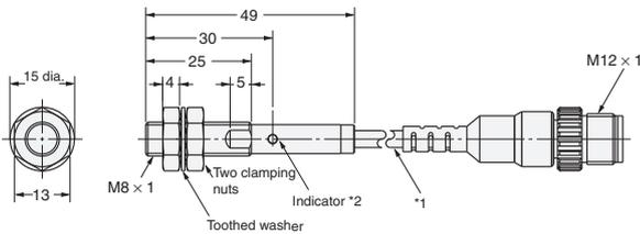
\*1. 4-dia. vinyl-insulated round cable (flame retardant), Standard length; 300 mm
