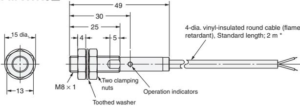
\* 4-dia. vinyl-insulated round cable with 2 conductors
