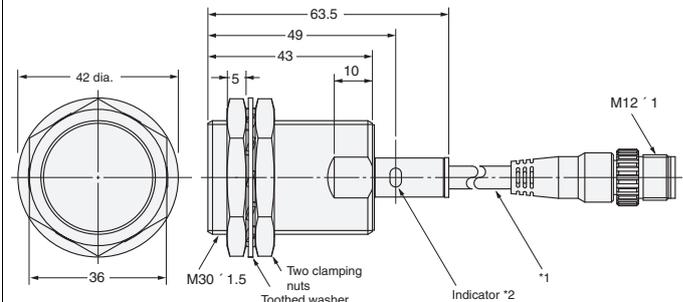
\*1. 6-dia. vinyl-insulated round cable (flame retardant), Standard length; 300 mm
