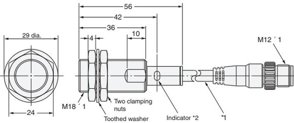
\*1. 6-dia. vinyl-insulated round cable (flame retardant), Standard length; 300 mm
