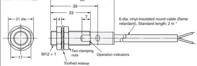
\* 6-dia. vinyl-insulated round cable with 2 conductors
