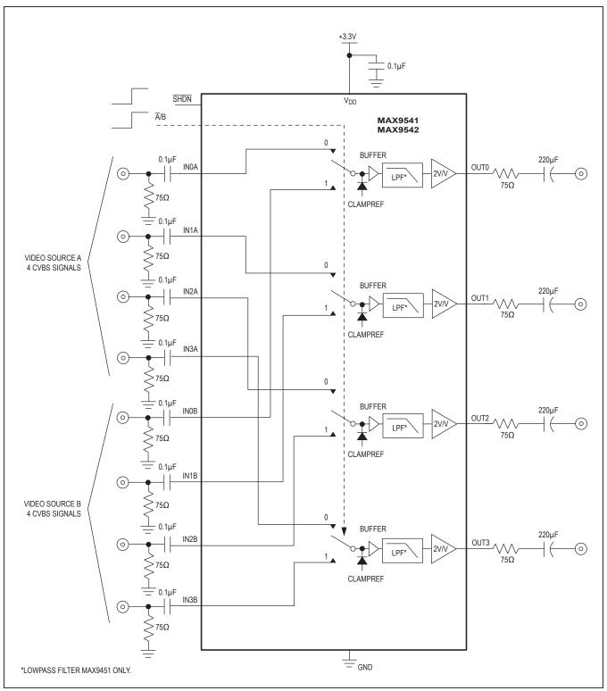
Figure 3. AC-Coupled Outputs
