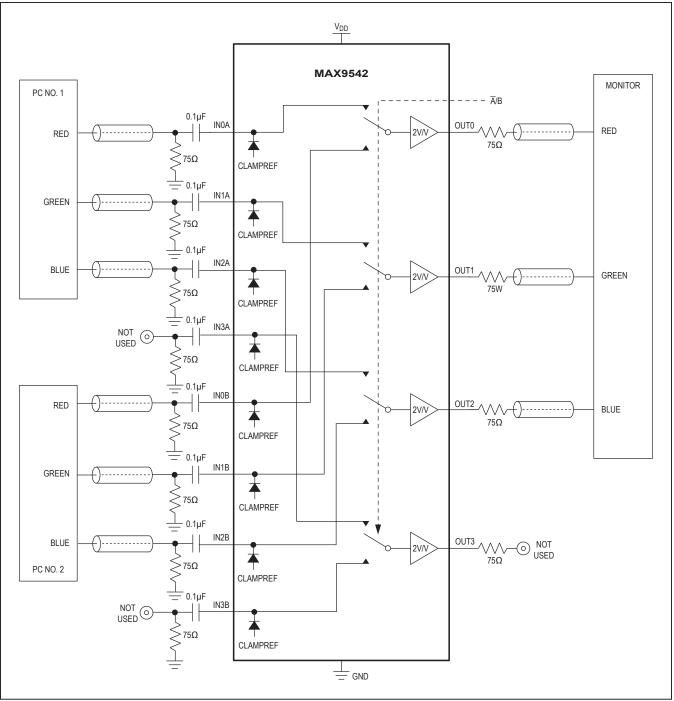
Figure 2. The MAX9542 Selecting Between Two VGA Sources
