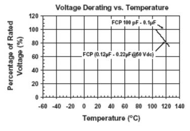
If the temperature on the surface of the capacitor is above 105°C, then the maximum voltage for FCP 50 Vdc ratings from .12 µF to .22µF must be derated linearly from full rated voltage at 105°C to 75% of the rated voltage at 125°C.
