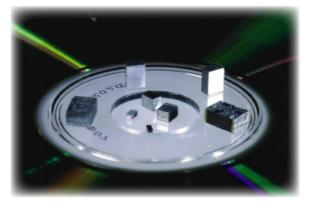
Type FCP stacked metallized polyphenelene sulfide (PPS) film capacitors offer high capacitance per unit volume, stable capacitance and DF over a wide temperature range, and excellent high frequency performance. Type FCP capacitors conform to standard EIA 0603, 0805, 1206, 1210, 1913 & 2416 surface mount case sizes and are packaged on tape and reel.
