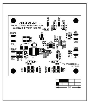
Figure 2. MAX16928 EV Kit Component Placement Guide— Component Side
