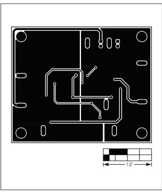
Figure 4. MAX16928 EV Kit PCB Layout—Solder Side
