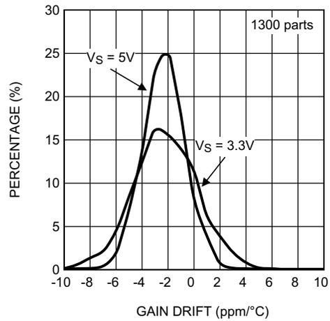
Figure 38. Gain Drift Distribution, 1300 Parts LMP8601 and LMP8601-Q1
