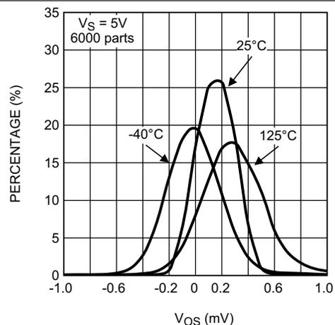
Figure 36.  $V_{\text{OS}}$  Distribution at  $V_S = 5\text{ V}$
