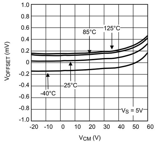
Figure 2.  $V_{\text{OS}}$  vs  $V_{\text{CM}}$  at  $V_S = 5\text{ V}$
