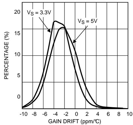
Figure 40. Gain Drift Distribution, 5000 Parts LMP8603 and LMP8603-Q1
