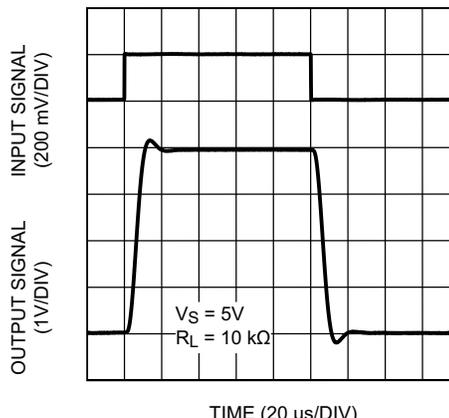
Figure 14. Step Response at  $V_S = 5\text{ V}$
