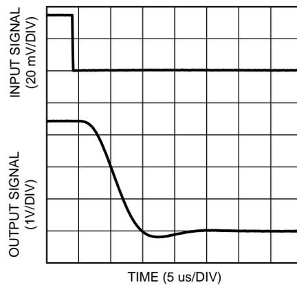
Figure 28. Settling Time (Falling Edge) at  $V_S = 5\text{ V}$
