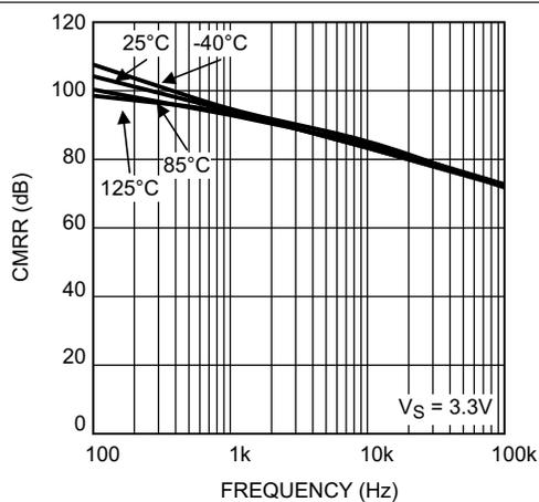
Figure 11. CMRR vs Frequency at  $V_S = 3.3\text{ V}$
