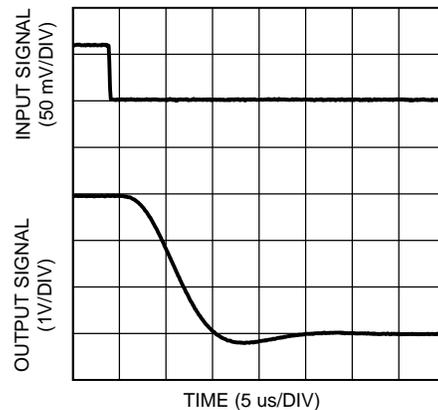
Figure 22. Settling Time (Falling Edge) at  $V_S = 5\text{ V}$
