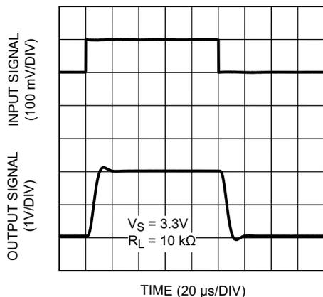
Figure 13. Step Response at  $V_S = 3.3\text{ V}$
