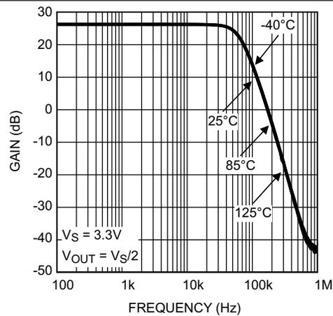
Figure 9. Gain vs Frequency at  $V_S = 3.3\text{ V}$
