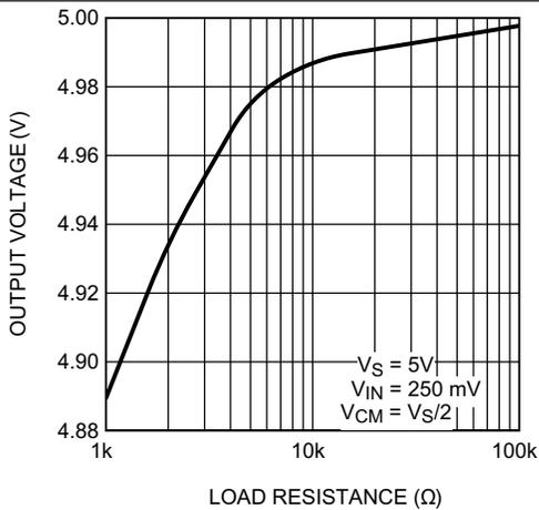
Figure 33. Positive Swing vs  $R_{\text{LOAD}}$   $V_S = 5\text{ V}$
