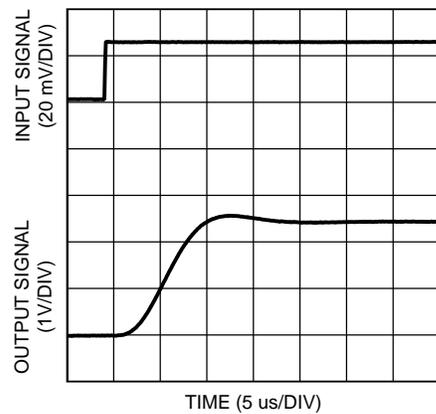
Figure 29. Settling Time (Rising Edge) at  $V_S = 3.3\text{ V}$
