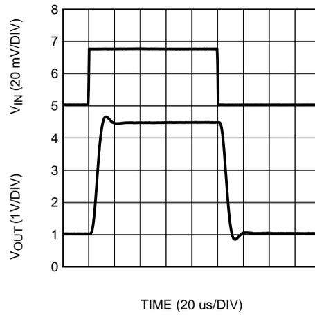
Figure 26. Step Response at  $V_S = 5\text{ V}$ ,  $R_L = 10\text{ k}\Omega$
