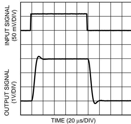
Figure 20. Step Response at  $V_S = 5\text{ V}$ ,  $R_L = 10\text{ k}\Omega$
