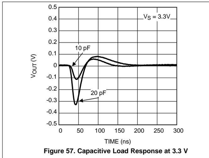
Figure 57. Capacitive Load Response at 3.3 V
