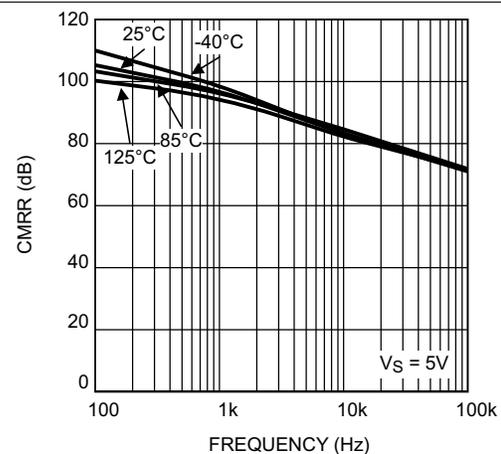
Figure 12. CMRR vs Frequency at  $V_S = 5\text{ V}$
