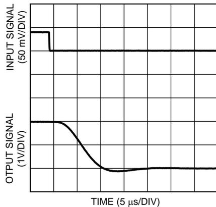
Figure 21. Settling Time (Falling Edge) at  $V_S = 3.3\text{ V}$
