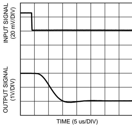
Figure 27. Settling Time (Falling Edge) at  $V_S = 3.3\text{ V}$
