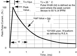
Fig. 2 - Pulse Waveform
