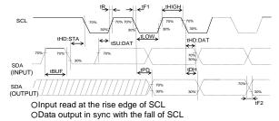
Figure 2-(a). Serial Input / Output Timing
