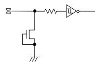
Figure 49. Input Pin Circuit Diagram
