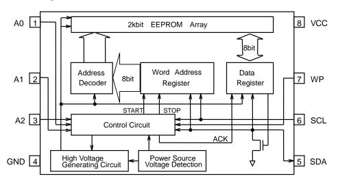
Figure 3. Block Diagram
