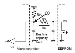
Figure 47. I/O Circuit Diagram
