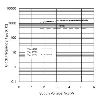
Figure 13. Clock Frequency vs Supply Voltage
