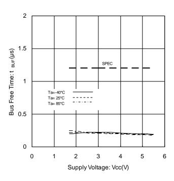
Figure 25. Bus Free Time vs Supply Voltage
