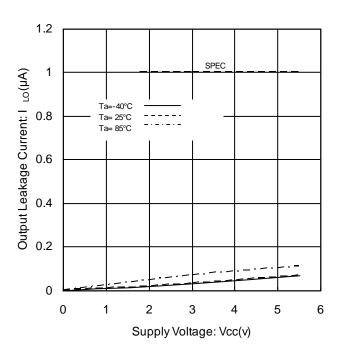
Figure 9. Output Leakage Current vs Supply Voltage (SDA)
