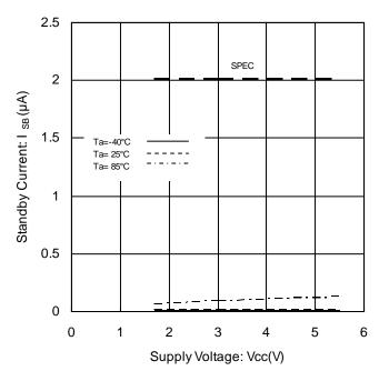
Figure 12. Standby Current vs Supply Voltage
