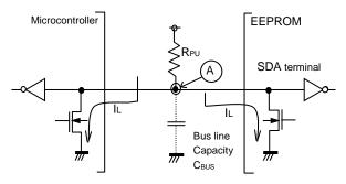
Figure 44. I/O Circuit Diagram
