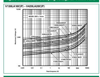
Figure 7. Maximum Clamping Voltage for 20mm Parts
