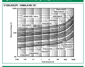
Figure 9. Maximum Clamping Voltage for Low Clamping Voltage Parts
