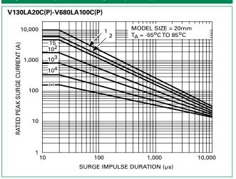
Note: Repetitive surge capability is qualified and tested based on 8/20us current waveform (not combination waveform) and UL1449 40.7.3 (Edition 4) test condition.
