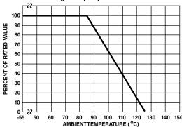
device. The operating values of a MOV need to be derated at high temperatures as shown above. Because varistors only dissipate a relatively small amount of average power they are not suitable for repetitive applications that involve substantial amounts of average power dissipation.
