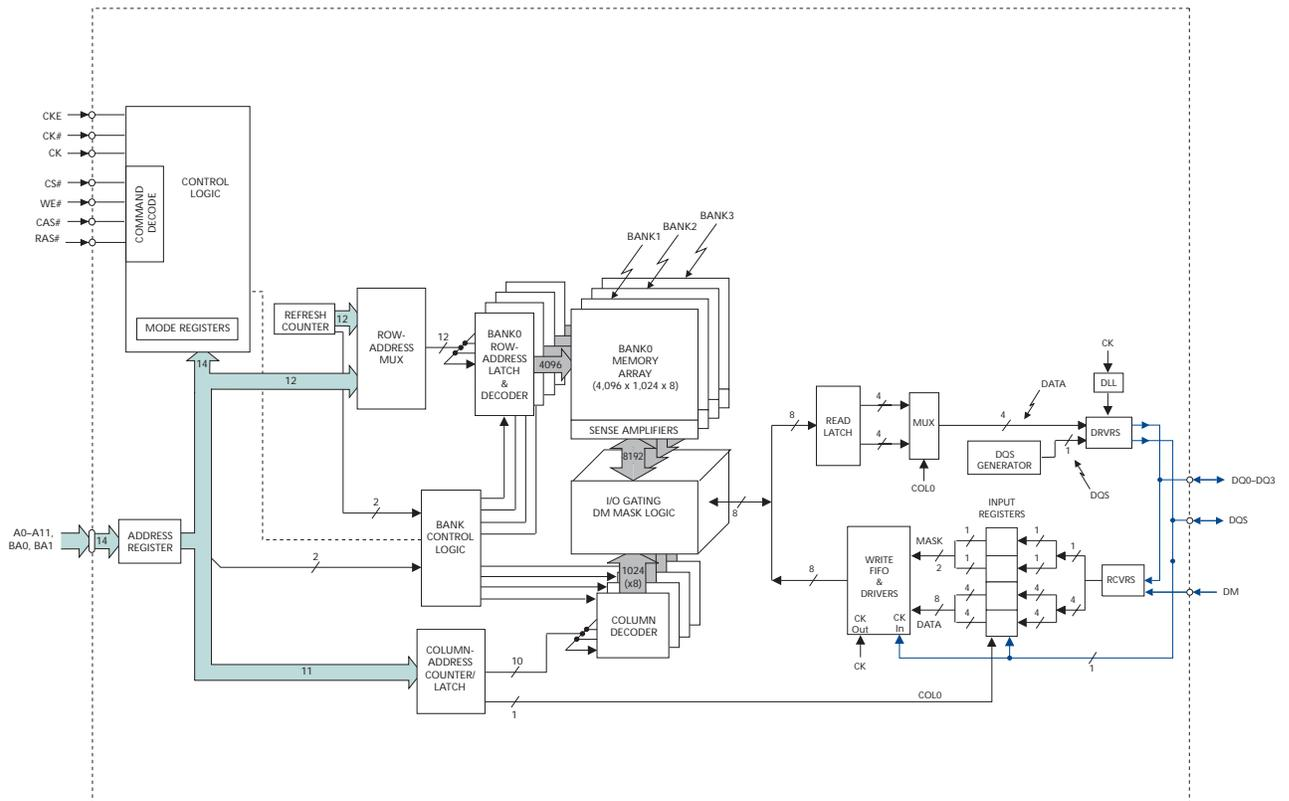
Figure 4: 16 Meg x 8 Functional Block Diagram
