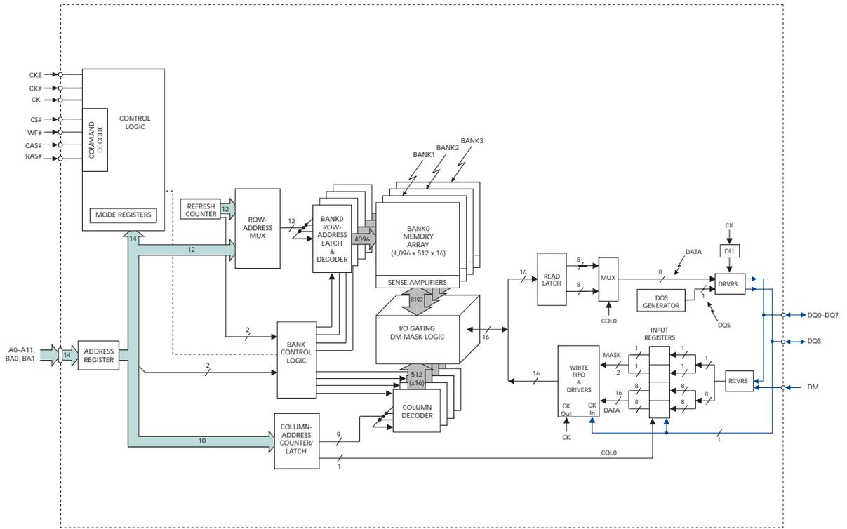
Figure 5: 8 Meg x 16 Functional Block Diagram
