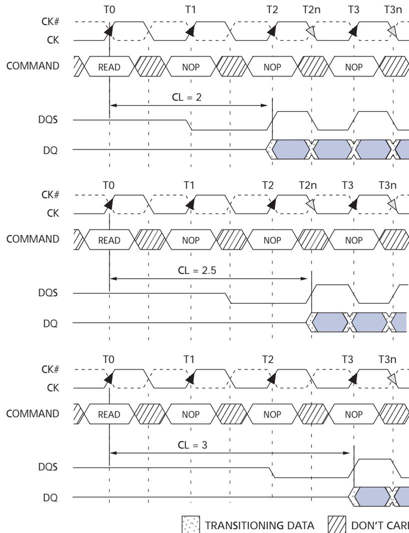
Note: BL = 4 in the cases shown; shown with nominal  $t_{AC}$ ,  $t_{DQSK}$ , and  $t_{DQSQ}$ .
