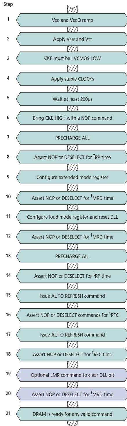
Figure 20: INITIALIZATION Timing Diagram
