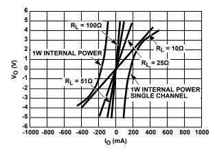
FIGURE 23. OUTPUT VOLTAGE AND CURRENT LIMITATIONS
