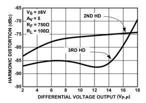
FIGURE 8. HARMONIC DISTORTION AT 2MHz
