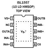
\*THERMAL PAD MUST BE CONNECTED TO NEGATIVE SUPPLY:  $V_{S_{\rm e}}$ . HMSOP PACKAGE CAN BE USED IN SINGLE SUPPLY APPLICATIONS ONLY.
