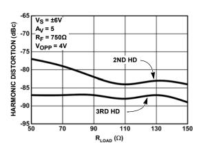
FIGURE 15. 2ND AND 3RD HARMONIC DISTORTION vs  $R_{LOAD}$  AT 10MHz
