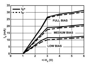
FIGURE 17. SUPPLY CURRENT vs SUPPLY VOLTAGE
