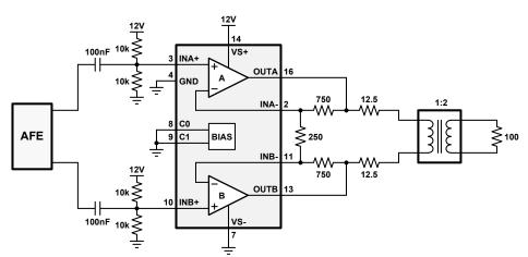
FIGURE 25. SINGLE SUPPLY OPERATION WITH INPUT COMMON-MODE BIASING
