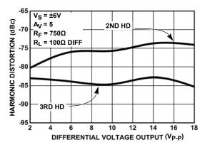
FIGURE 10. HARMONIC DISTORTION AT 3MHz
