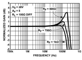
FIGURE 5. DIFFERENTIAL FREQUENCY RESPONSE WITH VARIOUS  $\mathbf{R_F}$  (FULL BIAS MODE)
