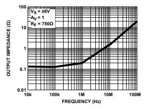
FIGURE 22. OUTPUT IMPEDANCE vs FREQUENCY
