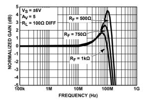
FIGURE 4. DIFFERENTIAL FREQUENCY RESPONSE WITH VARIOUS  $\mathbf{R_F}$  (LOW BIAS MODE)
