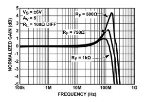
FIGURE 2. DIFFERENTIAL FREQUENCY RESPONSE WITH VARIOUS  $\mathbf{R_F}$  (FULL BIAS MODE)
