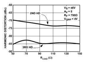
FIGURE 9. 2ND AND 3RD HARMONIC DISTORTION VS RLOAD AT
