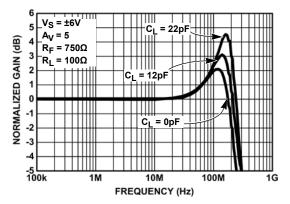
FIGURE 19. FREQUENCY RESPONSE vs VARIOUS C<sub>L</sub> (MEDIUM BIAS MODE)
