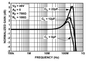
FIGURE 18. FREQUENCY RESPONSE WITH VARIOUS  $\mathbf{C_L}$  (FULL BIAS MODE)
