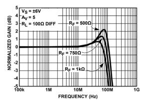
FIGURE 7. DIFFERENTIAL FREQUENCY RESPONSE WITH VARIOUS  $\mathbf{R_{F}}$  (LOW BIAS MODE)
