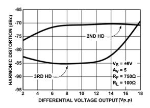
FIGURE 12. HARMONIC DISTORTION AT 5MHz
