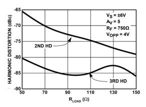
FIGURE 13. 2ND AND 3RD HARMONIC DISTORTION vs R<sub>LOAD</sub> AT
