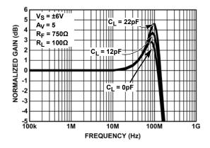
FIGURE 20. FREQUENCY RESPONSE WITH VARIOUS C<sub>L</sub> (LOW BIAS MODE)
