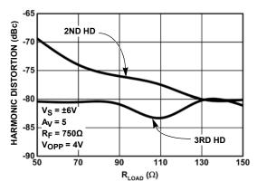
FIGURE 11. 2ND AND 3RD HARMONIC DISTORTION vs  $R_{LOAD}$  AT
