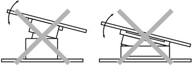
2. Keep the PC board warp no more than 0.03 mm in relation to the overall length of the connector.
