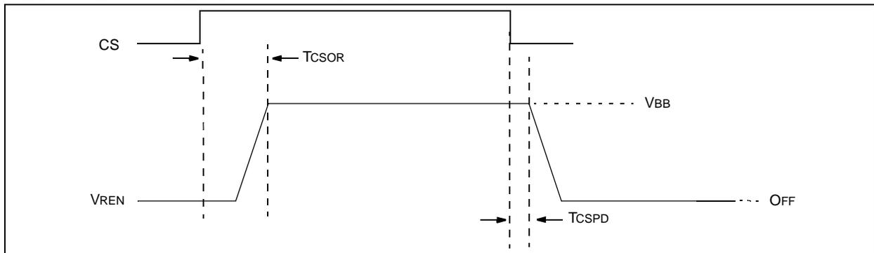
**FIGURE 2-6: BUS TO VREN WAKE TIMING DIAGRAM**
