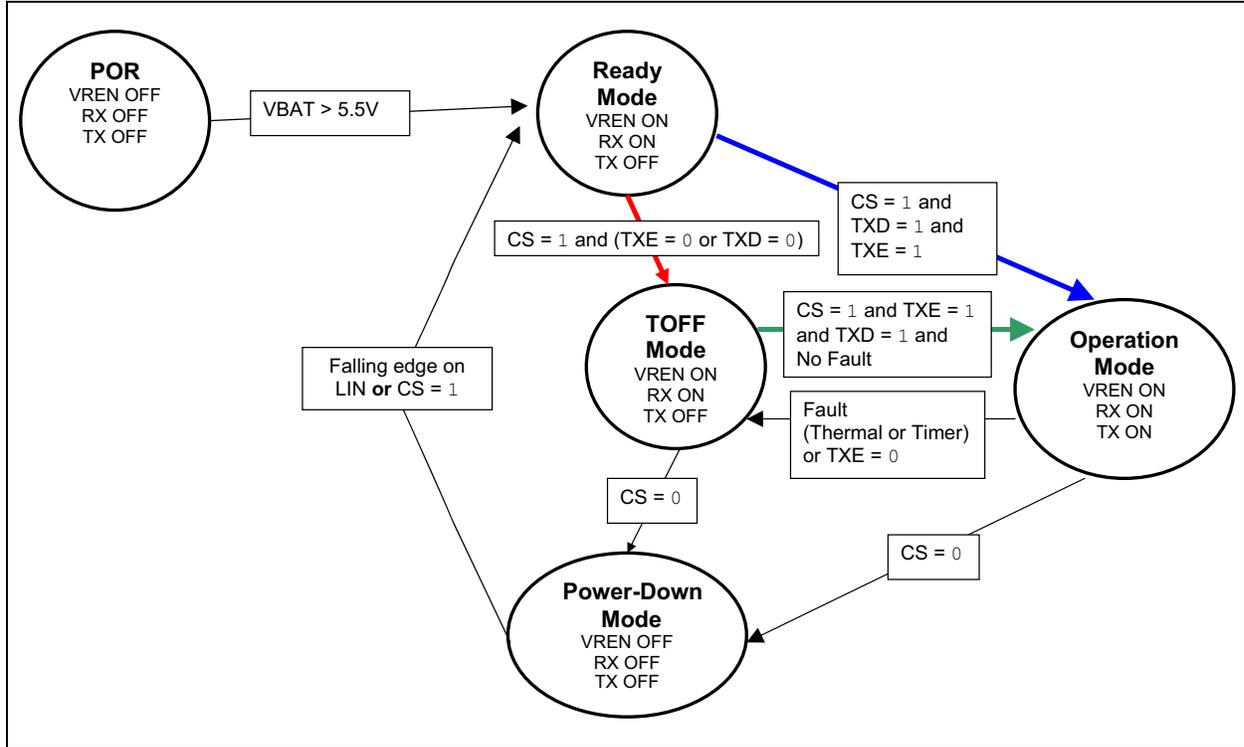
**Note:** While the MCP2003/4 is in thermal shutdown, TXD should not be actively driven high or it may power internal logic through the ESD diodes and may damage the device.
