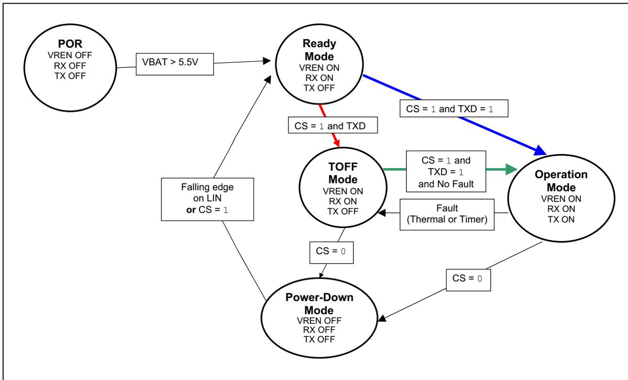
**FIGURE 1-3: OPERATIONAL MODES STATE DIAGRAM – MCP2004**
