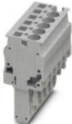
Plug, Connection method: Spring-cage connection, Number of positions: 13, Cross section: 0.08 mm<sup>2</sup> - 6 mm<sup>2</sup>, AWG: 28 - 10, Width: 80.6 mm, Height: 41.5 mm, Color: gray
