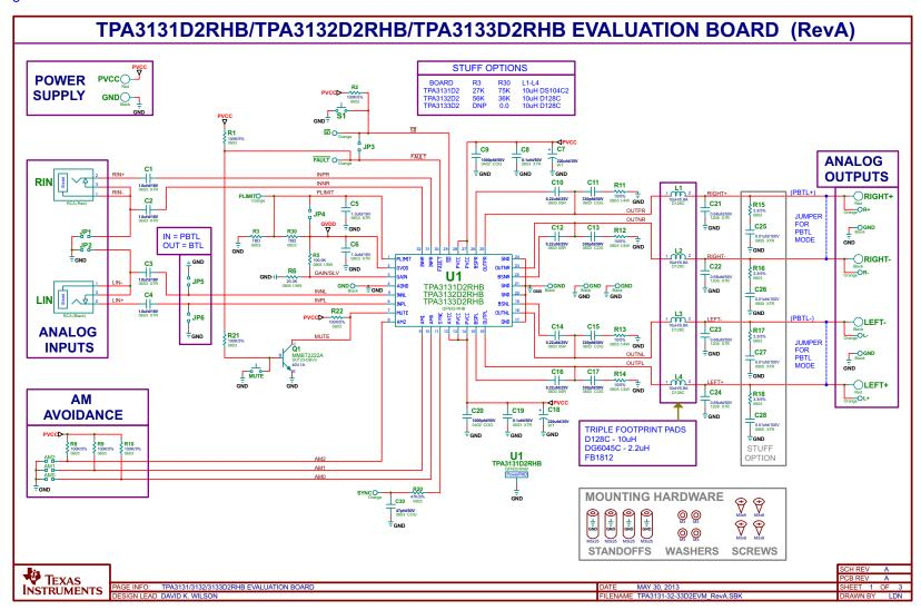
Figure 3. TPA3131D2EVM Schematic
