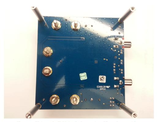
Figure 2. TPA3131D2EVM Audio Power Amplifier – Bottom View
