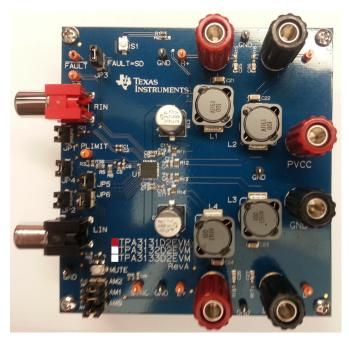
Figure 1. TPA3131D2EVM Audio Power Amplifier – Top View
