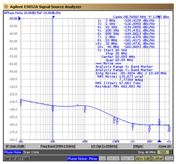
Figure 26. LMK04828 DCLKout2, VCO1, 245.76 MHz, Div12, LVPECL20 /w 240- $\Omega$  Emitter Resistor, DCLKoutX\_MUX=Divider, IDL=1, ODL=0, Balun = ADT2-1T
