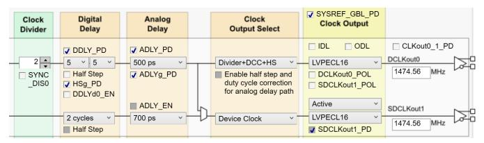
Figure 10. Setting Digital Delay, Clock Divider, Analog Delay and Output Format
