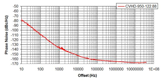
Figure 19. Crystek CVHD-950-122.88 MHz VCXO Phase Noise at 122.88 MHz
