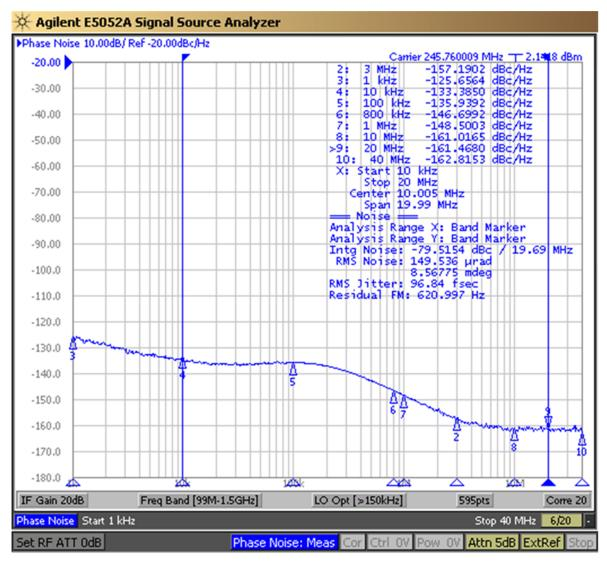
Figure 25. LMK04828 DCLKout2, VCO0, 245.76 MHz, Div10, LVPECL20 /w 240-Ω Emitter Resistor, DCLKoutX\_MUX=Divider, IDL=1, ODL=0, Single Ended
