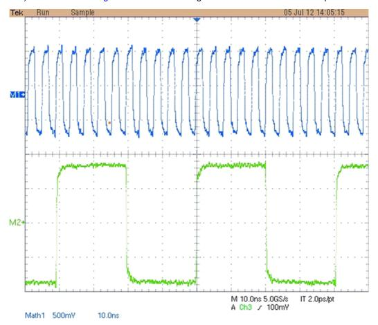
Figure 3. Continuous SYSREF Output
