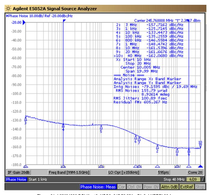
Figure 21. LMK04826 DCLKout2, VCO0, 245.76 MHz, Div8, LVPECL20 /w 240- $\Omega$  Emitter Resistor, DCLKoutX\_MUX=Divider, IDL=1, ODL=0, Single Ended
