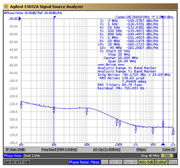
Figure 27. LMK04828 DCLKout2, VCO1, 245.76 MHz, Div12, LVPECL20 /w 240-Ω Emitter Resistor, DCLKoutX\_MUX=Divider, IDL=1, ODL=0, Single Ended
