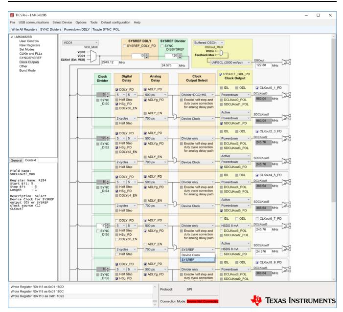
Figure 5. Clock Outputs Page Setup for SYSREF Output on SDCLKout7
