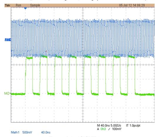
Figure 4. Pulsed SYSREF Output
