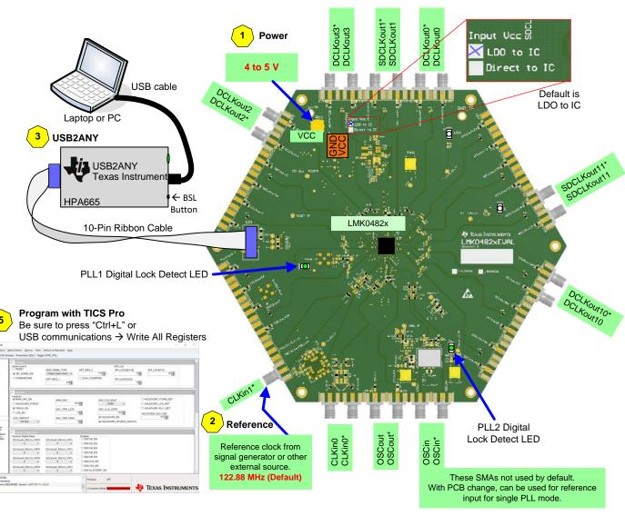
Figure 1. Quick Start Diagram
