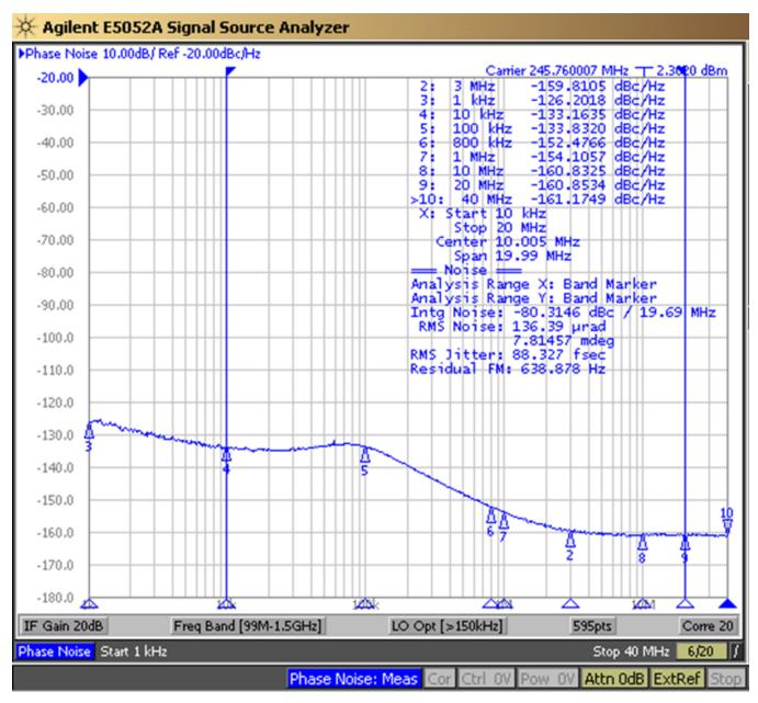
Figure 23. LMK04826 DCLKout2, VCO1, 245.76 MHz, Div10, LVPECL20/w 240-Ω Emitter Resistor, DCLKoutX\_MUX=Divider, IDL=1, ODL=0, Single Ended
