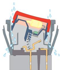
Current carrying parts are protected from moisture. Droplets which may enter the switch are channelled out through ports in the switch body.
