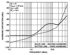
Figure 23. Harmonic Distortion vs. Frequency (SOIC)
