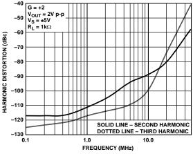
Figure 3. Harmonic Distortion vs. Frequency and Gain (SOIC)
