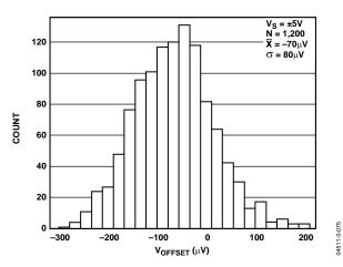
Figure 52. Input Offset Voltage Distribution
