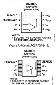
Figure 2. 8-Lead SOIC-EP (RD-8-1)
