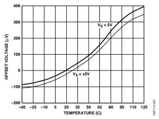
Figure 53. Input Offset Voltage vs. Temperature
