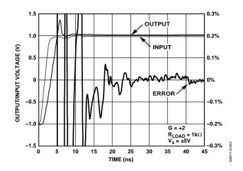
Figure 45. Short Term Settling Time (SOIC)
