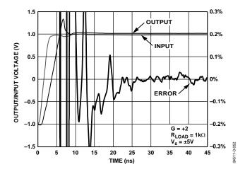
Figure 44. Short Term Settling Time (LFCSP)
