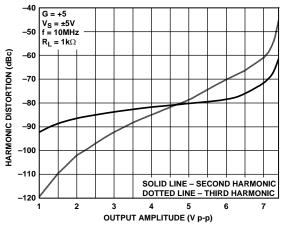
Figure 34. Harmonic Distortion vs. Output Amplitude (LFCSP)
