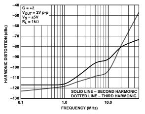
Figure 24. Harmonic Distortion vs. Frequency (SOIC)
