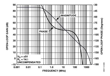
Figure 14. Open Loop Frequency Response
