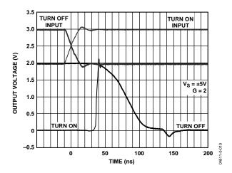
Figure 40. Disable/Enable Switching Speed
