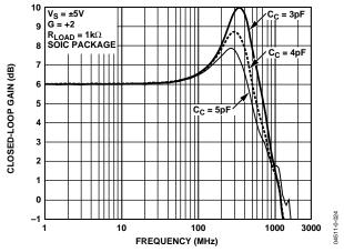
Figure 73. Frequency Response for Various Values of  $C_C$
