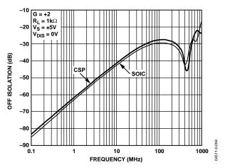
Figure 21. Off Isolation vs. Frequency
