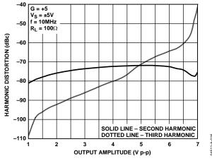
Figure 30. Harmonic Distortion vs. Output Amplitude (SOIC)
