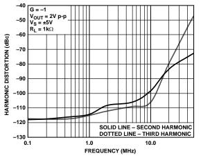
Figure 25. Harmonic Distortion vs. Frequency (SOIC)
