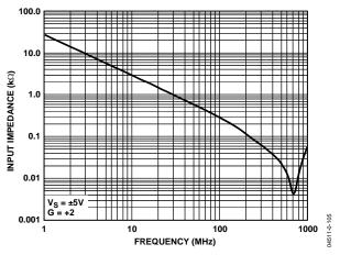
Figure 18. Input Impedance vs. Frequency
