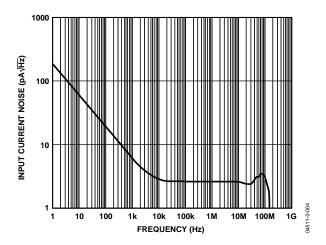
Figure 48. Input Current Noise vs. Frequency (DISABLE = Open)
