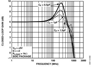
Figure 71. Frequency Response for Various Values of C<sub>F</sub>
