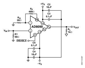
Figure 66. Amplifier Configuration for LFCSP and SOIC Packages, Gain = +20
