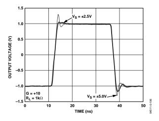
Figure 41. Large Signal Transient Response vs. Supply Voltage (LFCSP)
