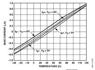
Figure 57. Input Bias Current vs. Temperature ( $\overline{DISABLE}$  Pin = +V<sub>S</sub>)
