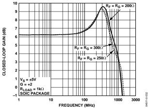
Figure 68. Frequency Response for Various Values of R<sub>F</sub> and R<sub>G</sub>
