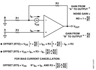
Figure 75. Op Amp Total Offset Voltage Model
