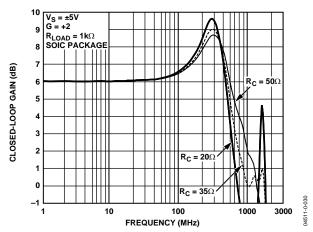
Figure 70. Frequency Response for Various Values of Rc
