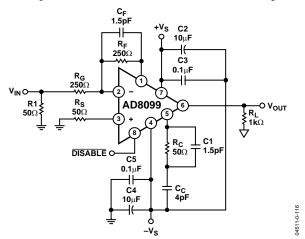
Figure 60. Amplifier Configuration for SOIC Package, Gain = -1
