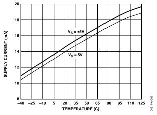
Figure 56. Supply Current vs. Temperature
