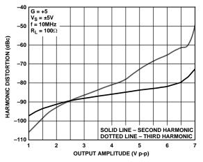
Figure 33. Harmonic Distortion vs. Output Amplitude (LFCSP)
