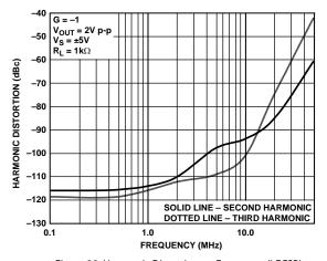
Figure 28. Harmonic Distortion vs. Frequency (LFCSP)
