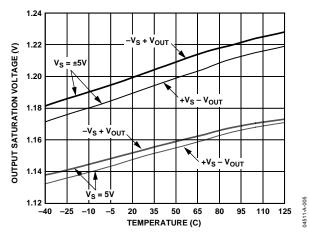
Figure 55. Output Saturation Voltage vs. Temperature
