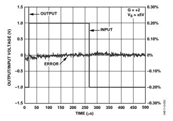
Figure 46. Long Term Settling Time
