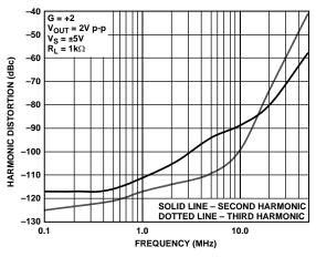
Figure 27. Harmonic Distortion vs. Frequency (LFCSP)
