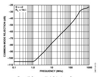
Figure 47. Common-Mode Rejection vs. Frequency
