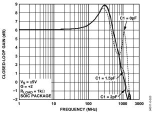
Figure 72. Frequency Response for Various Values of C1
