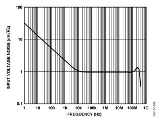
Figure 49. Input Voltage Noise vs. Frequency
