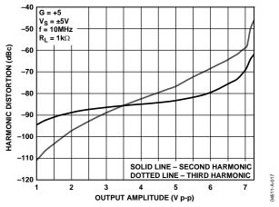
Figure 31. Harmonic Distortion vs. Output Amplitude (SOIC)
