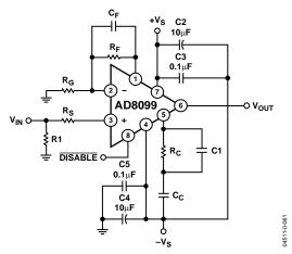
Figure 59. Wideband Noninverting Gain Configuration (SOIC)
