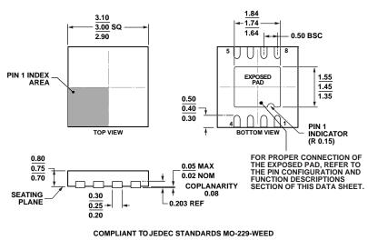
Figure 78. 8-Lead Lead Frame Chip Scale Package [LFCSP] 3 mm × 3 mm Body and 0.75 mm Package Height (CP-8-13) Dimensions shown in millimeters
