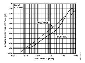
Figure 50. Power Supply Rejection vs. Frequency
