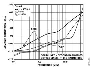
Figure 22. Harmonic Distortion vs. Frequency
