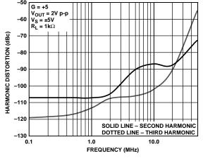
Figure 26. Harmonic Distortion vs. Frequency (LFCSP)
