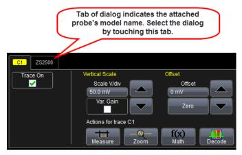
The probe can be controlled through the oscilloscope graphical user interface. When connected, a Probe dialog appears behind the corresponding channel dialog. Refer to your oscilloscope's manual for specific operation instructions.
