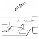
The straight tip is rugged and designed for general probing. Fits in either probe socket. (PK-ZS-001)
