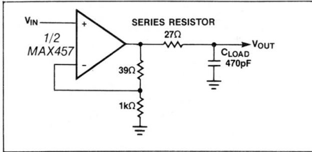
Figure 2. Isolating a Capacitive Load
