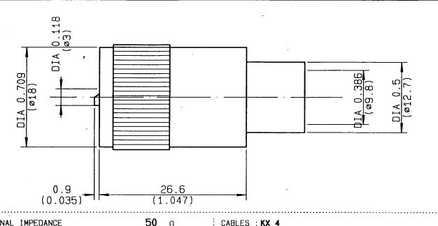
NOMINAL IMPEDANCE DC-0.5 FREQUENCY RANGE GHz -55/+155 TEMPERATURE RATING 1.3 +0 x F(GHz)Maxi V.S.W.R 0.5√F(GHz) dB Maxi RF INSERTION LOSS 750 Veff Maxi **VOLTAGE RATING** DIELECTRIC WITHSTANDING VOLTAGE 2000 Veff Mini INSULATION RESISTANCE 5000 MΩMini Atm.cm<sup>3</sup>/s HERMETIC SEAL
