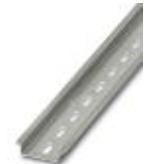
DIN rail, material: steel galvanized and passivated with a thick layer, perforated, height 7.5 mm, width 35 mm, length: 2000 mm
