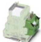
V8-OUTPUT adapter for eight 6.2 mm PLC interfaces (1 PDT, etc./see "Supplementary Products"). 14-pos. flat-ribbon cable connection for the PLC system cabling, control logic: Minus switching
