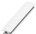
Zack marker strip, Strip, white, labeled, can be labeled with: Plotter, Printed horizontally: Consecutive numbers 1 - 10, 11 - 20, etc. up to 491 - 500, Mounting type: Snap into tall marker groove, for terminal block width: 6.2 mm, Lettering field: 6.15 x 10.5 mm
