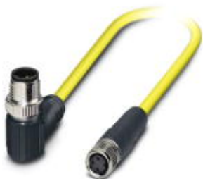
Sensor/actuator cable, 3-position, PVC, yellow, shielded, Plug angled M12 SPEEDCON, coding: A, on Socket straight M8, cable length: 1.5 m
