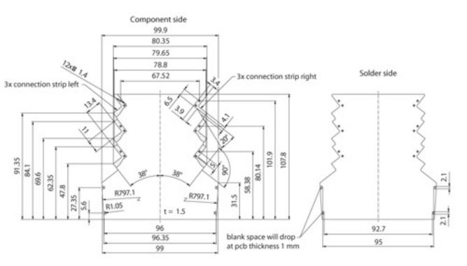
non dimensioned radii max R1 inhibited surface
